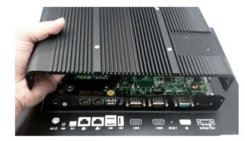
2. Remove the Fieldbus I/O cover.
