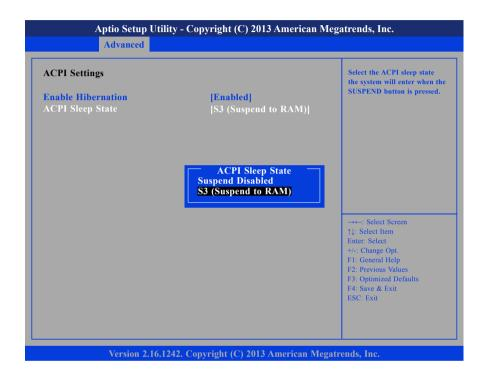
Select the highest ACPI sleep state the system will enter when the suspend button is pressed. The options are Suspend Disabled and S3 (Suspend to RAM).
