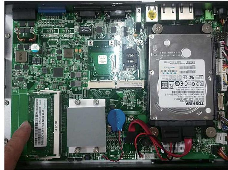
4. Push the module down until the clips on both sides of the socket lock into position. You will hear a distinctive “click” sound, indicating the module is correctly locked into position.
