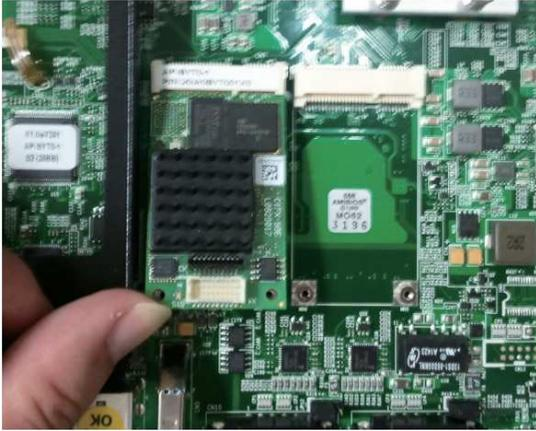
8. Secure the module with mounting screws.
