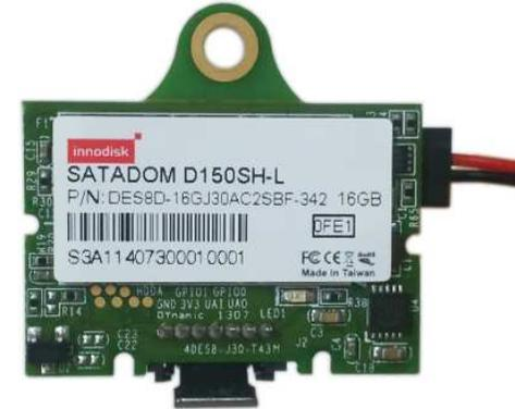
5. Install the module to the SATA port via the connector at the solder side of the module and then secure the module using the mounting screw you removed in step 1.
