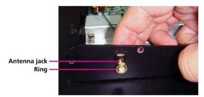
8. Connect external antennas to the antenna jacks.
