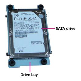
5. Align the mounting holes that are on the sides of the SATA drive with the mounting holes on the drive bay and then use the provided mounting screws to secure the drive in place.
