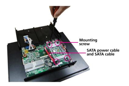
3. Remove the drive bay. The drive bay is used to hold a SATA hard drive.
