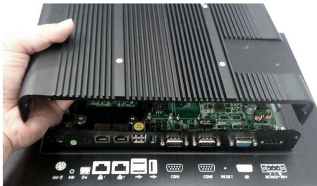
2. Remove the Fieldbus I/O cover.
