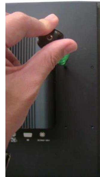
3. Wire the power adapter cabling into the cable opening on the bracket, then place the adapter inside the bracket.
