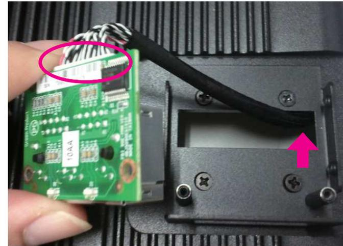
**Dual RJ45 Connector Board**
