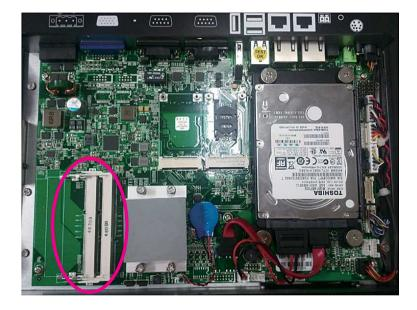
3. Insert the module into the socket at an approximately 30 degrees angle. Apply firm even pressure to each end of the module until it slips into the socket. The gold-plated connector on the edge of the module will almost completely disappear inside the socket.
