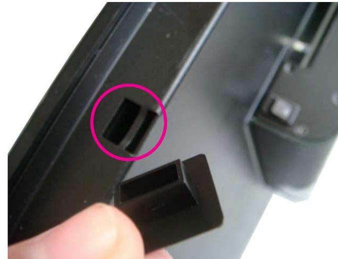
2. Insert the hole block into the opening until it is pushed in completely.
