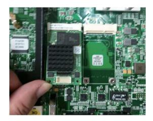
8. Secure the module with mounting screws.
