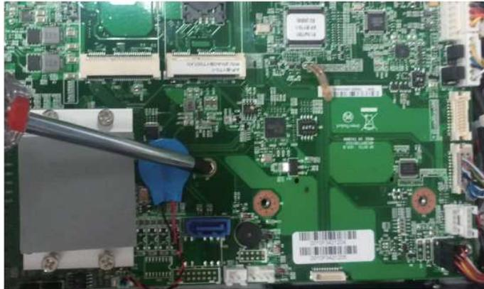
2. The SATA DOM package includes a supporting stud. The stud is used to stabilize the SATA DOM module.
