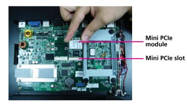
2. Secure the module with mounting screws.
