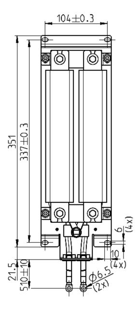
General tolerances according to ISO 2768-cL Dimensions in mm
