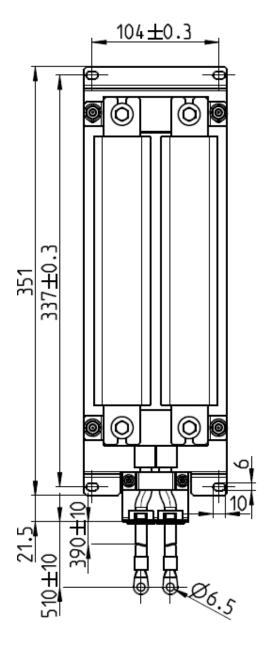
General tolerances according to ISO 2768-cL Dimensions in mm
