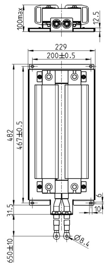
General tolerances according to ISO 2768-cL Dimensions in mm
