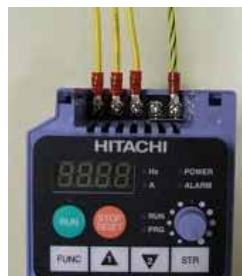
Input wiring for 3-phase input (models -NFU, -HFEF, -HFU)
