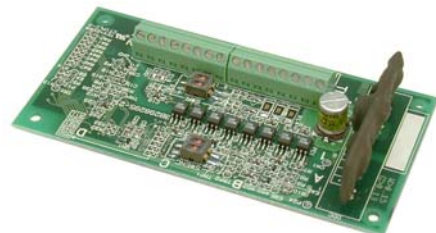
Expansion Card - Encoder Input
