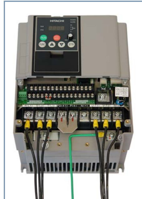
To power source To chassis ground To motor
