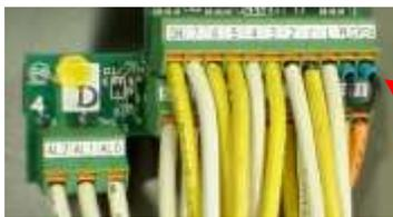
NOTE: in above pictures, the length of ground cable is not suitable. To avoid pulling the cable unintentionally, you need to cut the ground cable to an appropriate length for the distance to the inverter's grounding terminal and the size of the terminal block, and crimp the cable to the crimp terminal before using.
