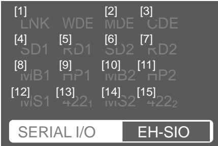
Figure. 8.1 Order of the LED check
