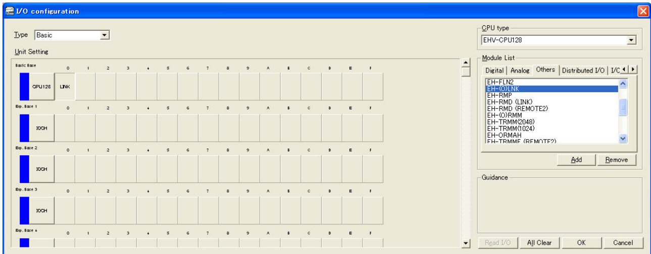
Figure1.1.1 I/O assignment for link module with Control Editor (in the case of "LINK")
