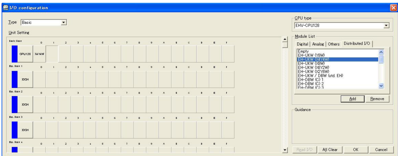
Figure1.1.2 I/O assignment for link module with Control Editor (in the case of "X4Y4W")
