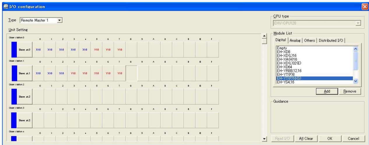
Figure 4.5.8 I/O assignment example of remote I/O after the replacement (Assignment of Figure 4.5.7 configuration example by control editor)
