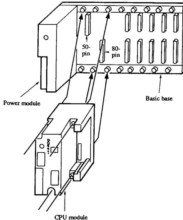
**Figure 12.4 How to mount the CPU Module**
