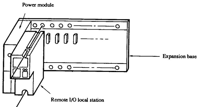
**Figure 12.6 Mounting a Remote I/O Local Station**
