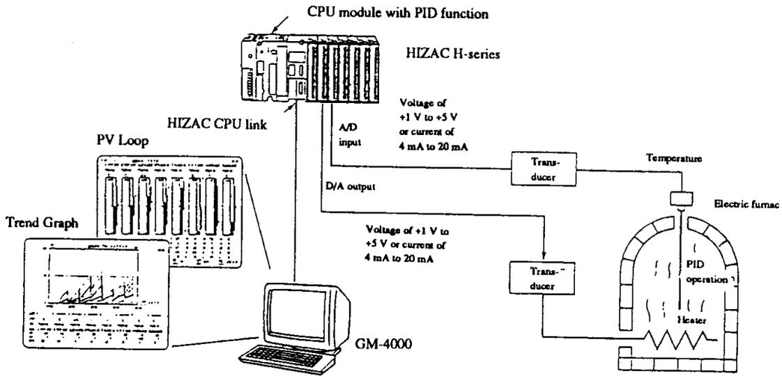
Electric furnace temperature control (example)
