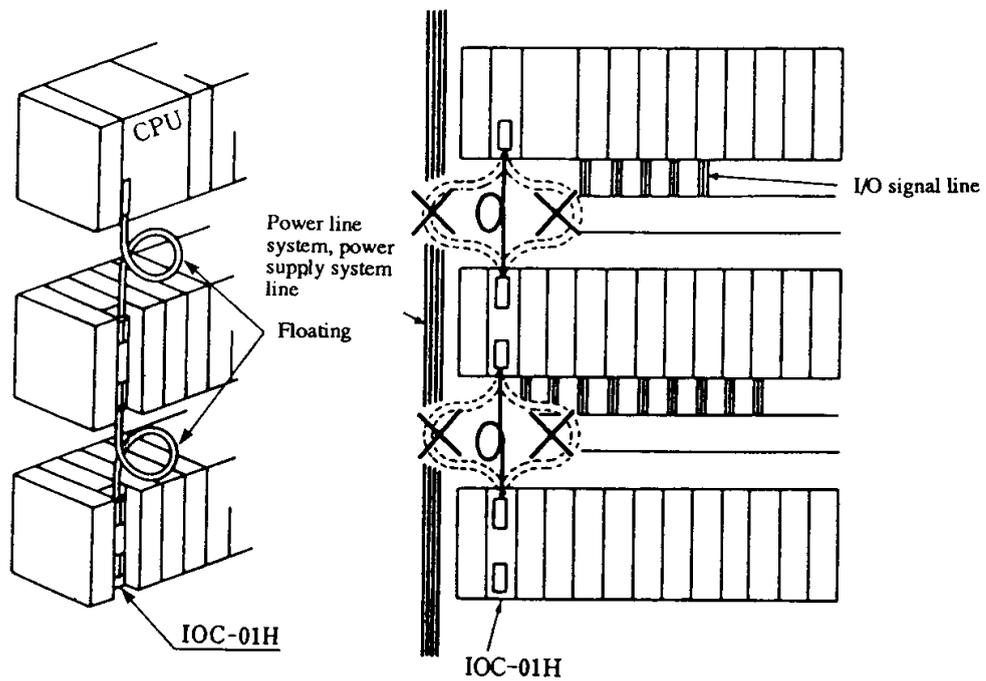
Be sure to separate each additional cable (CBL-□□H, CBE-□□H) from the power line, I/O signal line, and power supply system line.
