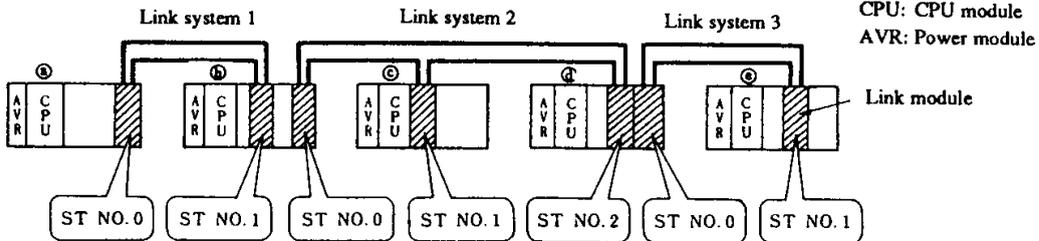
The link area of each CPU is divided into a transmission area and reception area. In the transmission area, data of the ST (station) No. of the self station is set. This data is transferred successively to each link area in the same link. Namely, the CPUs in the same link have the same data.
