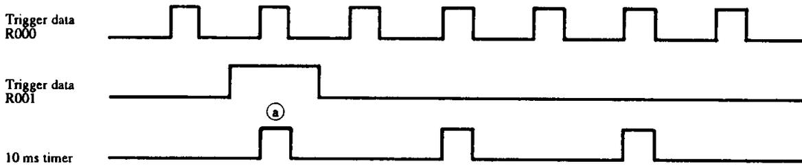
When the 10-ms timer is started, the trigger circuit monitor function checks the I/O which is set in the trigger requirements. When the I/O matches with the trigger data, the function samples the I/O data which is used in the specified circuit. In the above case, when the trigger data bit I/O R000 and R001 are in the ON state or at [a], the function samples the I/O data which is used in the set circuit.
