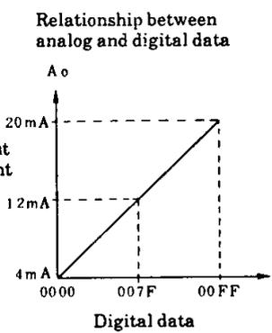
If the external load resistance exceeds 510 Ω, the 20 mA maximum current requirements may not be satisfied.
