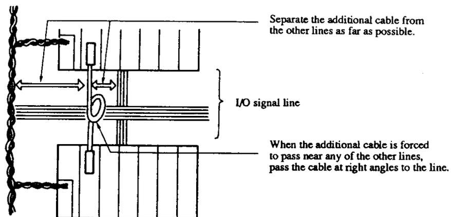
Figure 12.9 Distribution Example of an Additional Cable
