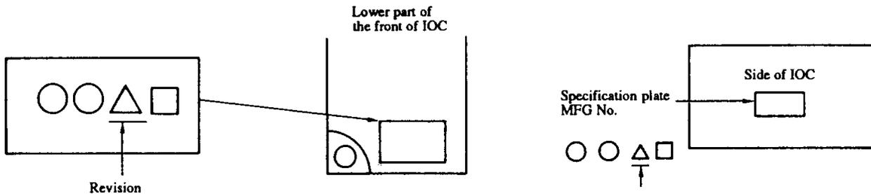
The revision is displayed on the lower part of the front of IOC-01H or on the specification plate. Be sure to check it. When there is no display on the lower part of the front of IOC-01H, the revision is E or a previous release. It cannot be used for H-2002 and H-702.
