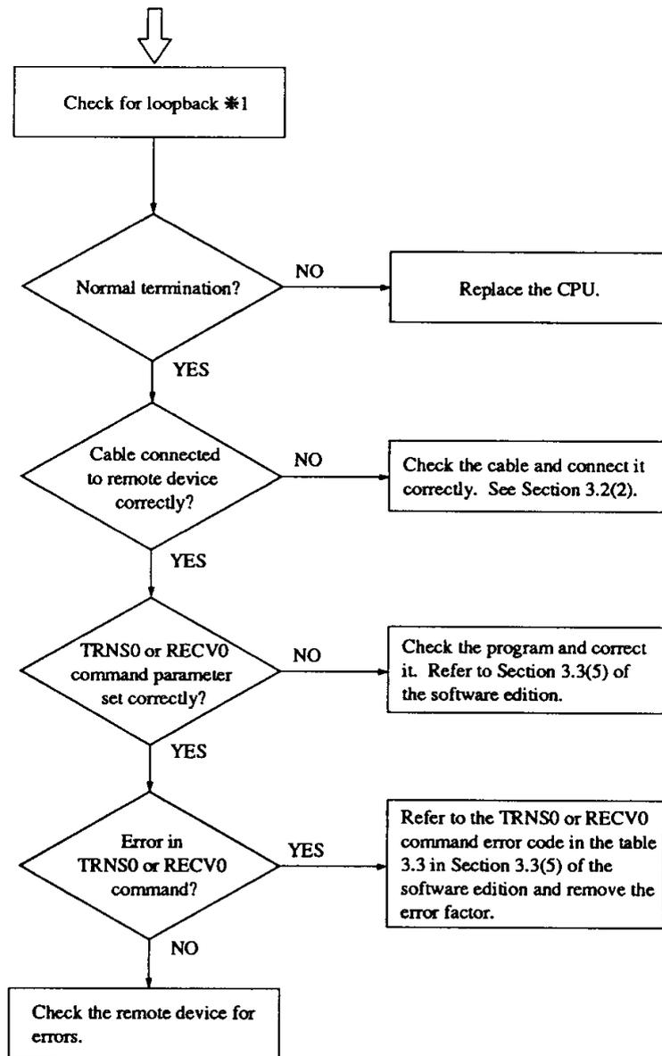
**\*1:** The loopback check is a check for separating an error in the CPU module and an error in the cable or remote device from each other on a hardware basis. It does not check the TRNS0 and RECV0 commands (rationality of the user program). For the loopback check method, see the next and subsequent pages.
