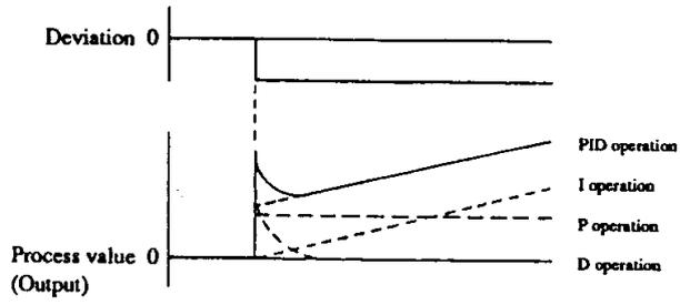
PID operation on step-like deviation
