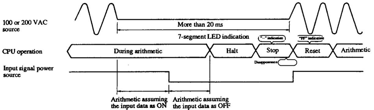
A power failure of each power module of the H-series is detected by a voltage drop of the internal DC source. Therefore, the holding time varies with the number of mounted modules and arithmetic may be continued for 20 to 350 ms.
