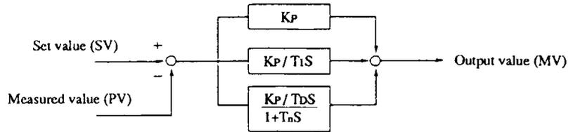
Block diagram of PID operation
