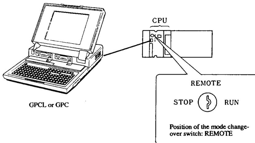
For debug running of the program, the graphic input device (GPCL) is used. Set the mode changeover switch of the CPU to REMOTE. The following two statuses of the CPU are available for debug.
