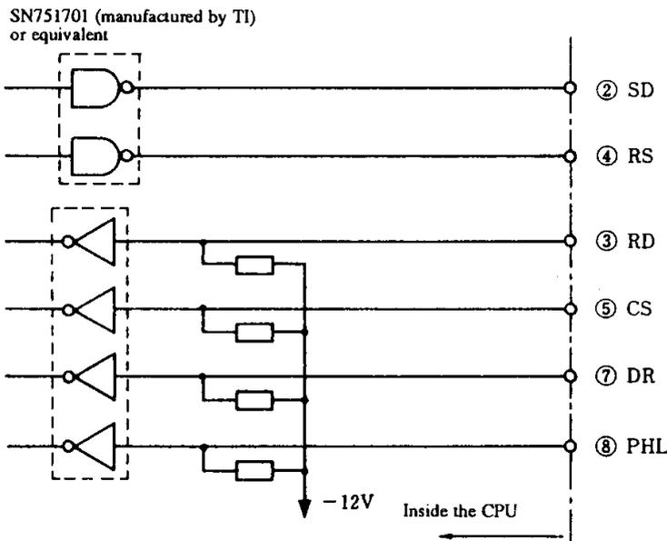
RS-232C interface circuit (peripheral port)
