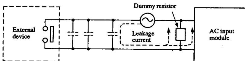
[3] Method that the external power source is connected to the external device
