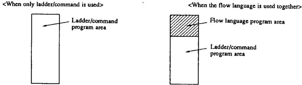
When the flow language is used, the user program area is allocated using the graphic programming console (GPCL01H). For the allocation method, refer to the software edition (CPU Setting) of the instruction manual of the graphic programming console (GPCL01H).
