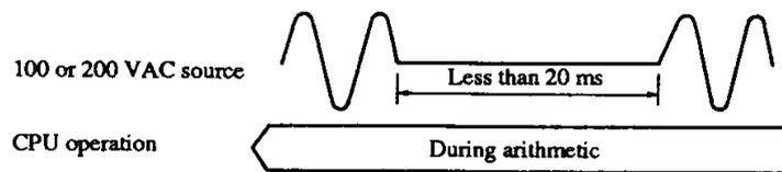
**Note 1:** Hold the input signal power source when the CPU performs the operation continuously. When it is not held, the CPU performs arithmetic assuming the input data as OFF. Note that when the CPU particularly performs arithmetic for changing the power failure storage content by an input signal, the CPU may change the power failure storage content by mistake due to instantaneous power failure.
