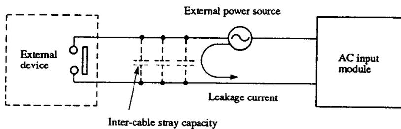
This phenomenon is that even if the contact of the external device is opened, a leakage current flows by the inter-cable stray capacity and a voltage is generated at the input terminal of the AC input module.
