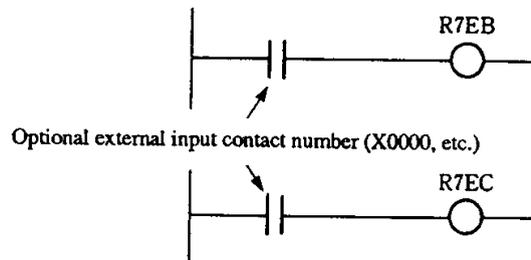
As a method for setting 1 in the special internal output, a method using a program as shown on the right or a method of forced set or reset by the peripheral equipment is available.
