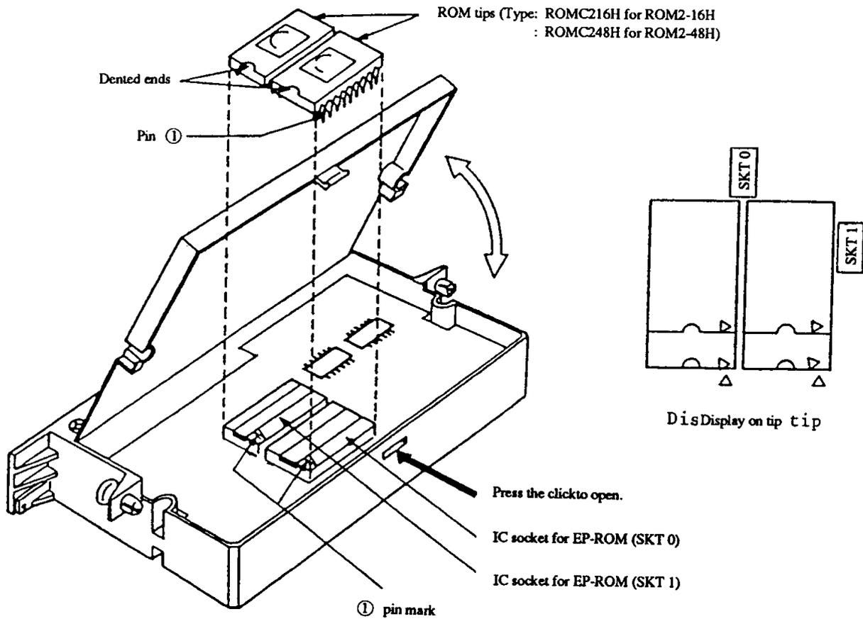
(ii) Check the following after installation of the ROM tips
