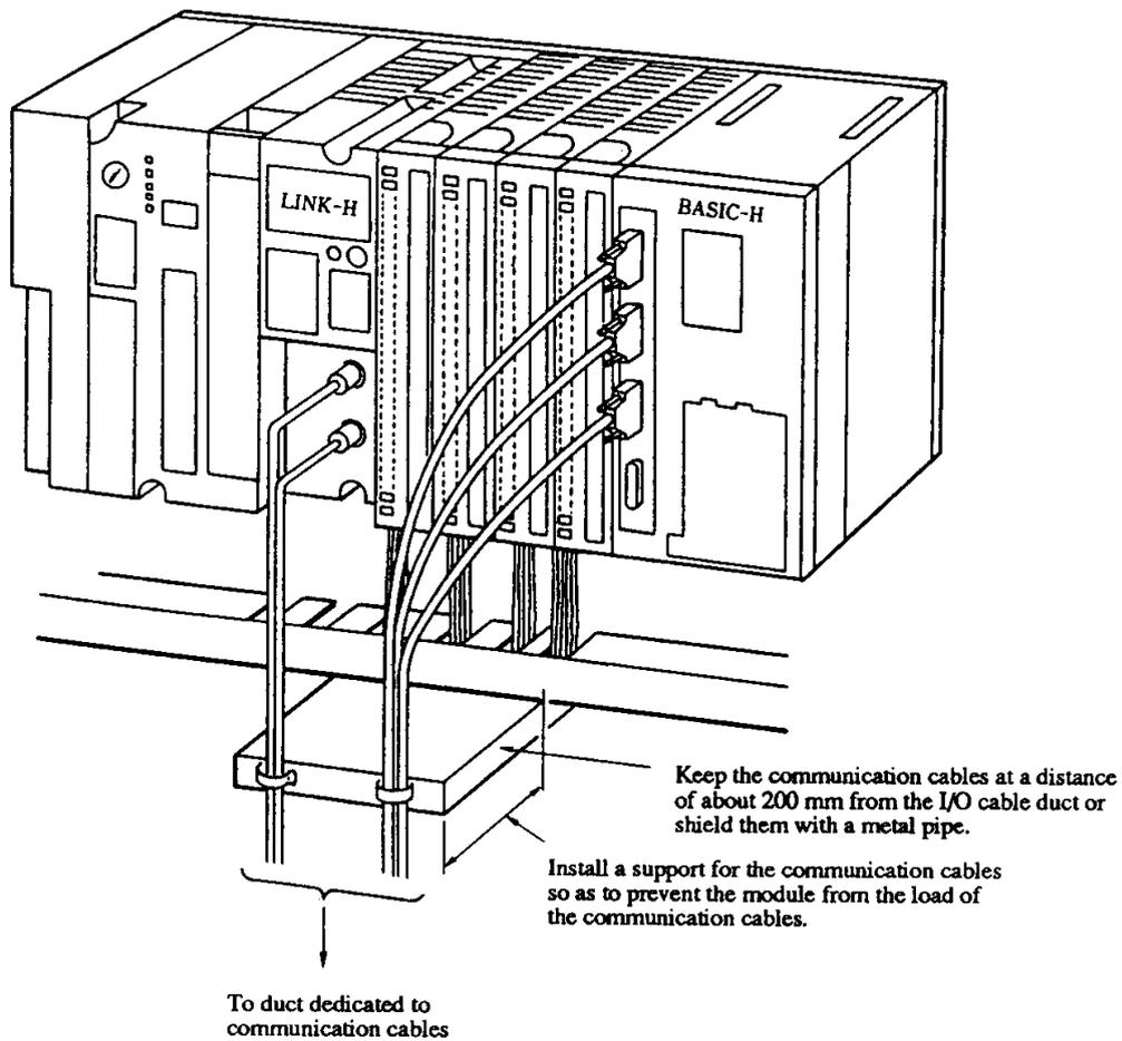
Figure 12.10 Communication Module Cable Distribution Example
