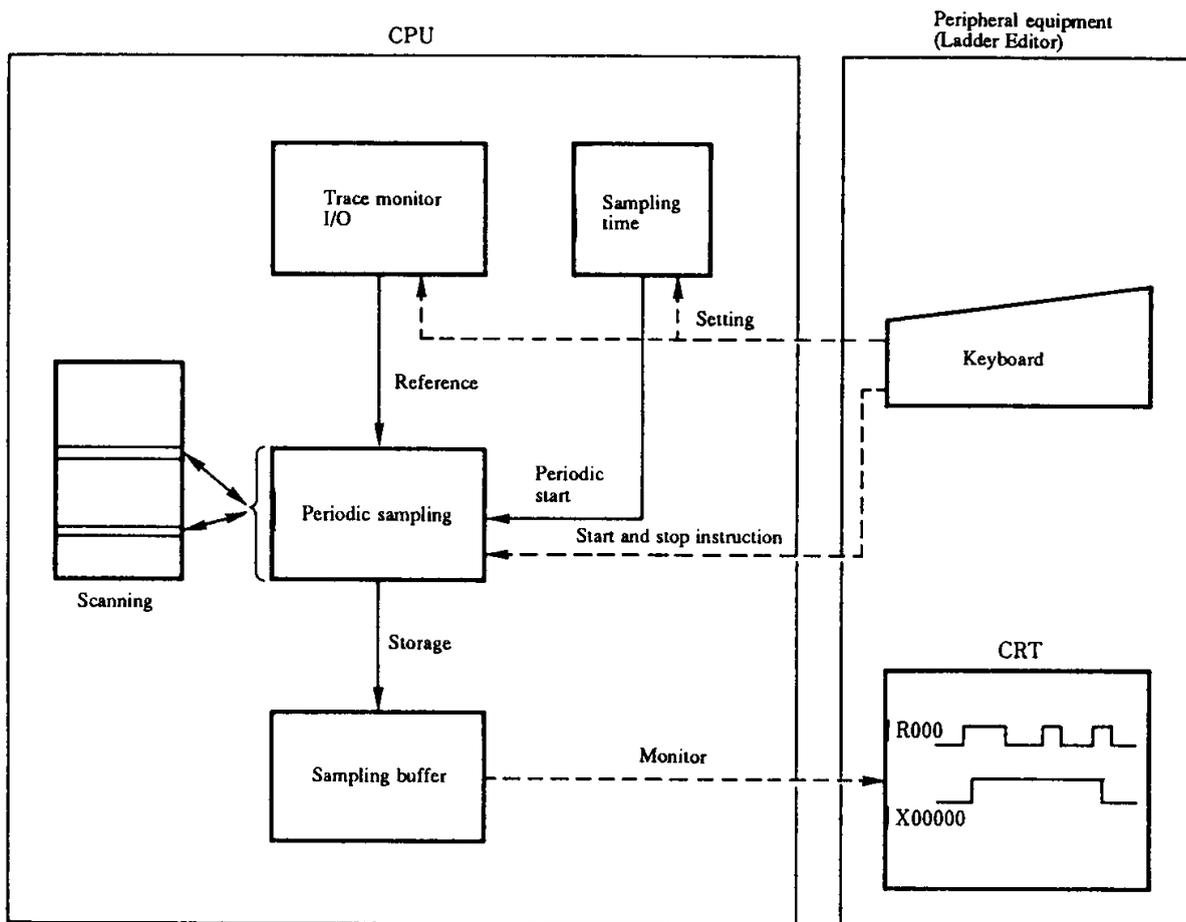
**Note:** When data is being monitored by the continuous time chart function or continuous trace function, the trace status may be changed to the STOP mode. The reason is that the data amount becomes larger than the data amount which is stored in the sampling buffer by the CPU within a specified time and no data can be written into the sampling buffer any more.
