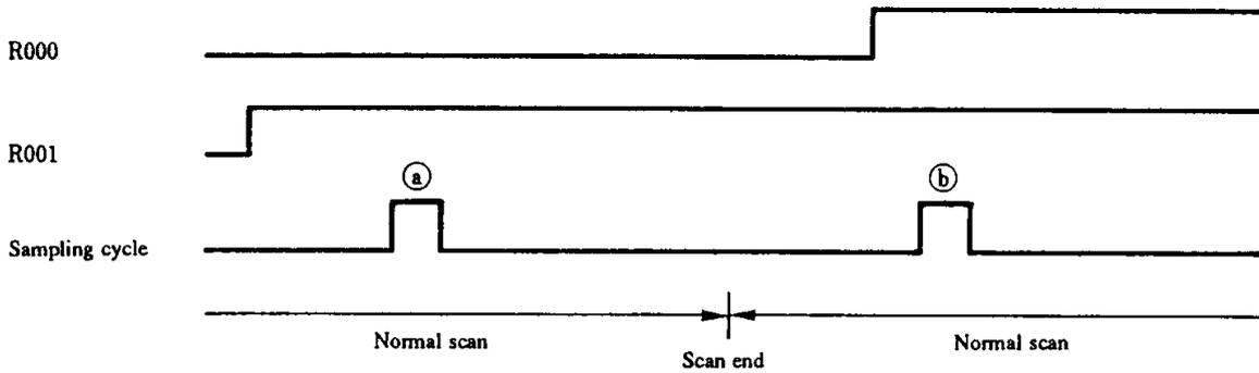
When the sampling trace instruction provided in the ladder program is executed at [a] or [b], the CPU instruction trace function samples the set I/O data.
