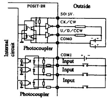
※1: The external supply current is a current flowing into the S0 terminal.
