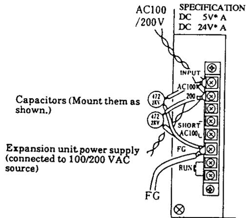
Part A: Wiring details at power module terminal block
