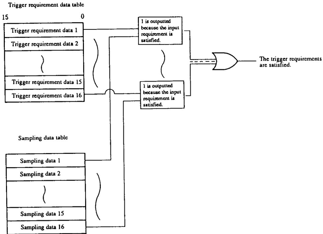
The trigger OR requirements mean that when there is at least one set of the trigger requirement data which is set in each I/O and the sampling data corresponding to the I/O which match with each other, the trigger requirements are satisfied.
