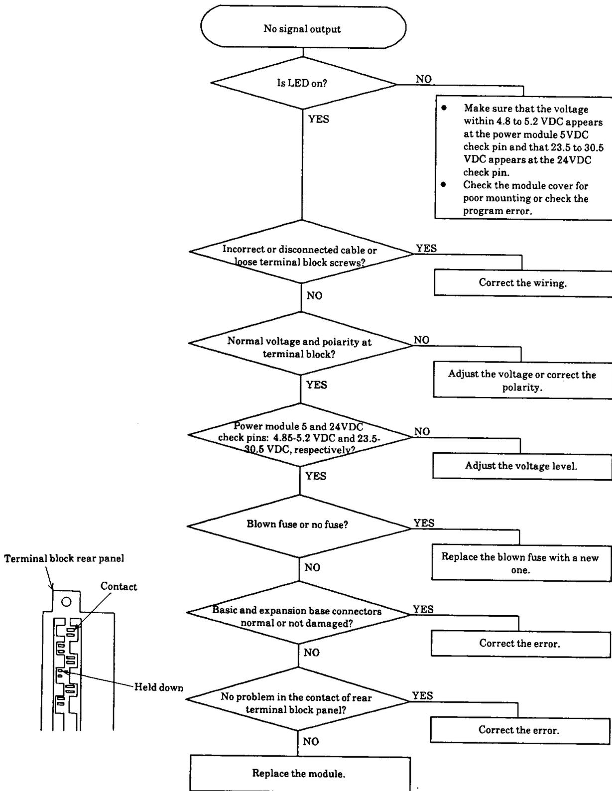
(b) Check during normal signal input but I/O assignment error exists
