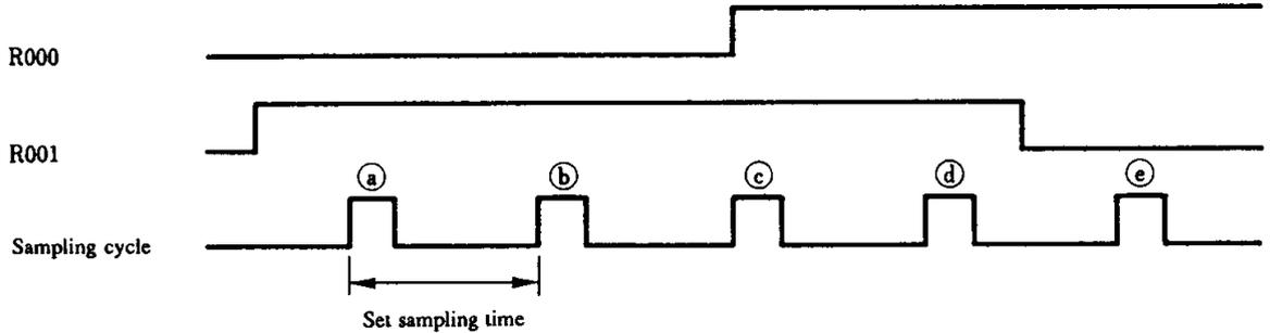
The sampling cycle is determined by the set sampling time. At [a] and [b] during data sampling, R000 is OFF, though R001 is ON and data is sampled.
