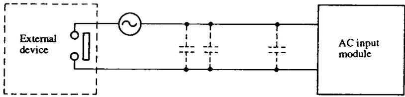
(c) Effect of leakage current
