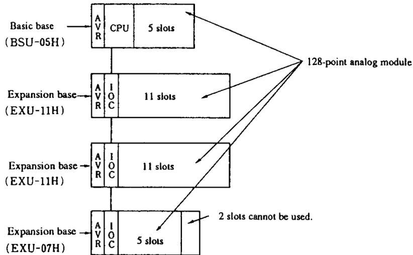
**(2) When the external I/O area and remote I/O area are used (Concept on a remote I/O system)**
