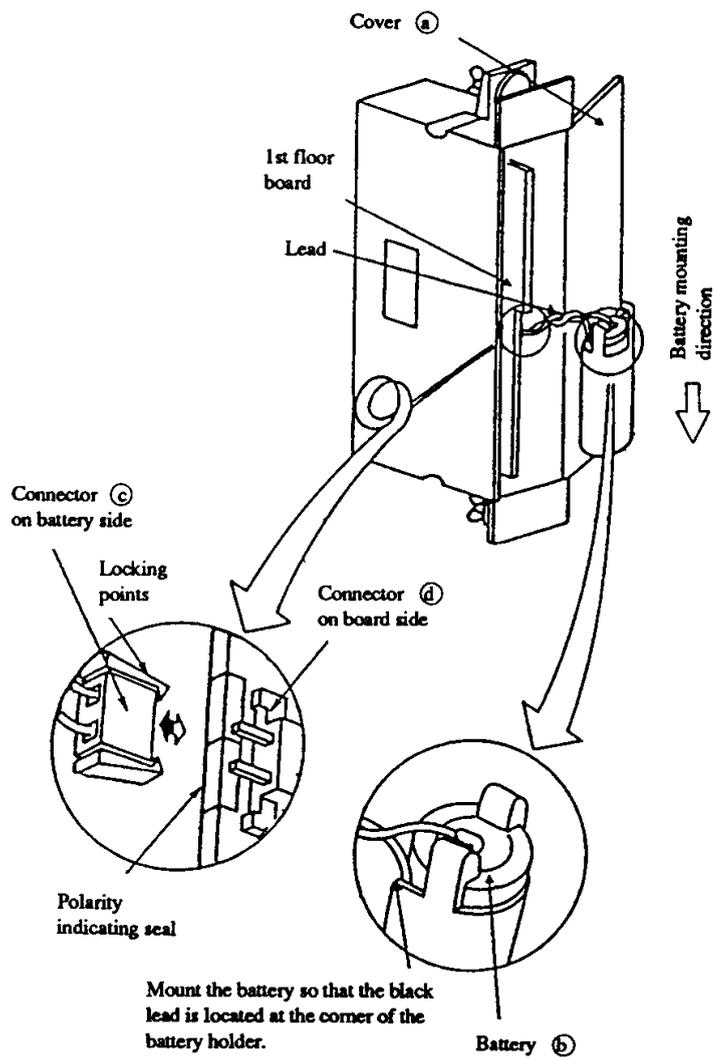
[2] Replacing the battery
