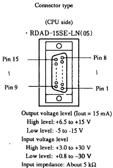
**(2) Specification of the general purpose (non-protocol) port (Valid only when the CPU type is CPU2-\*\*H)**
