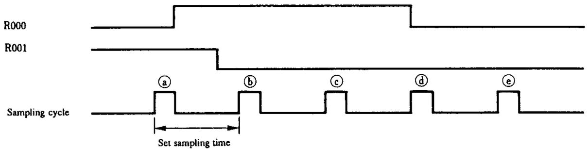
The sampling cycle is determined by the set sampling time. At [b] during data sampling, the trigger requirements are satisfied and the trigger time chart function is stopped.
