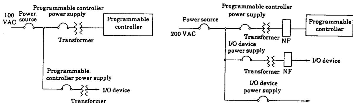
Figure 12.7 Example of Power Supply System Diagram
