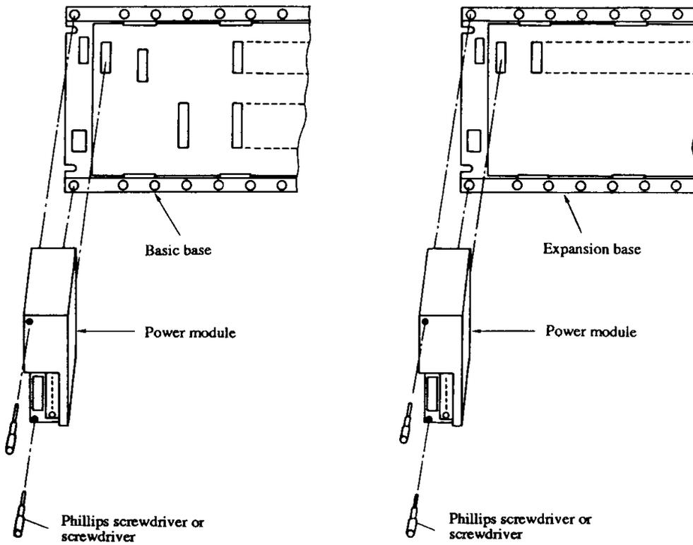
Figure 12.3 How to mount the Power Module
