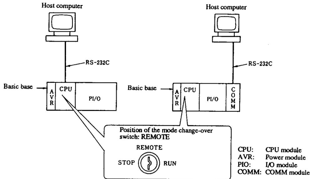
When the host computer issues a task code (CPU control code) to the PC, the user program runs or stops.
