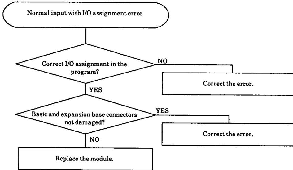
(c) Check during normal input with LED being off
