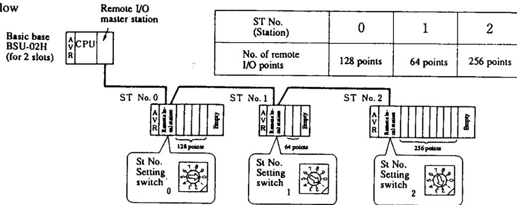
Control status of the number of I/O points of the remote I/O master station
