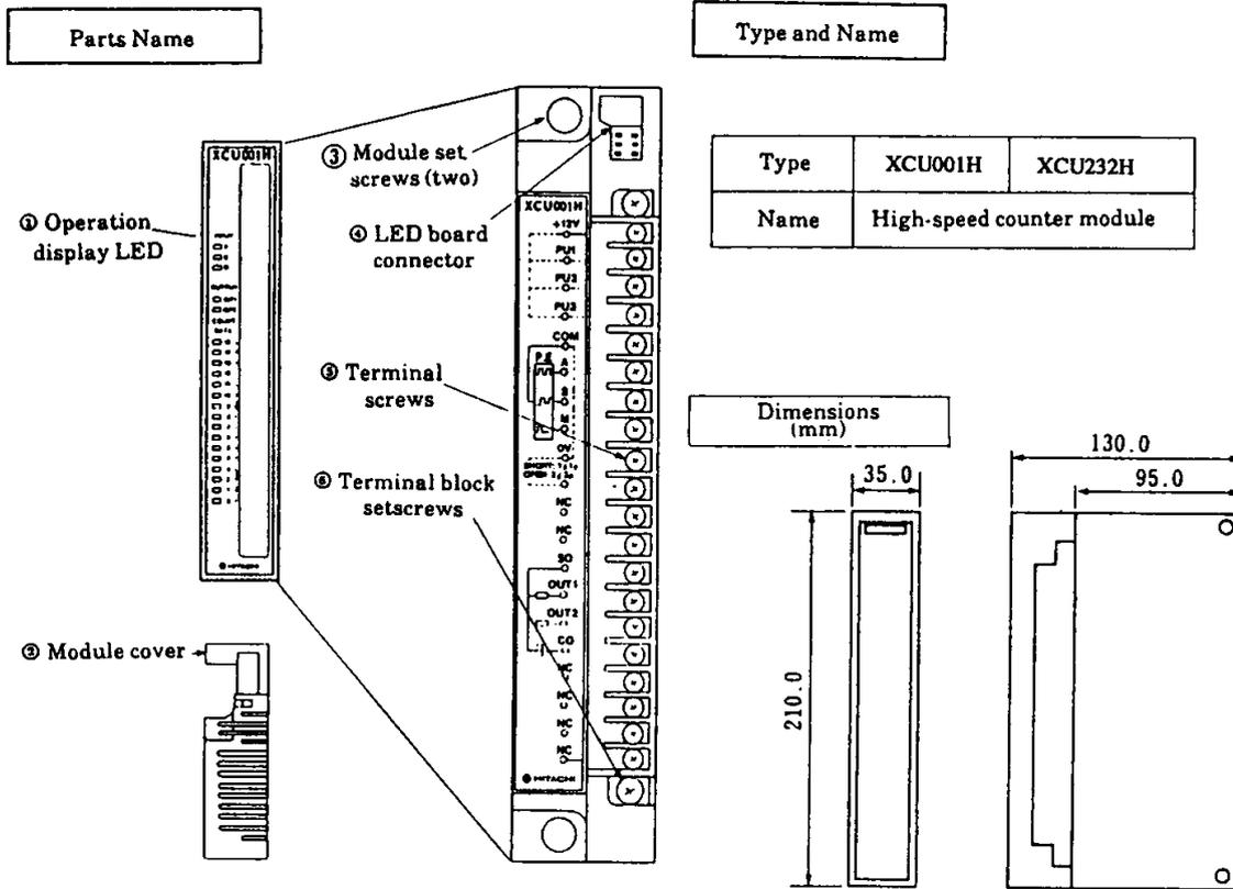
(a) High-speed counter module specifications
