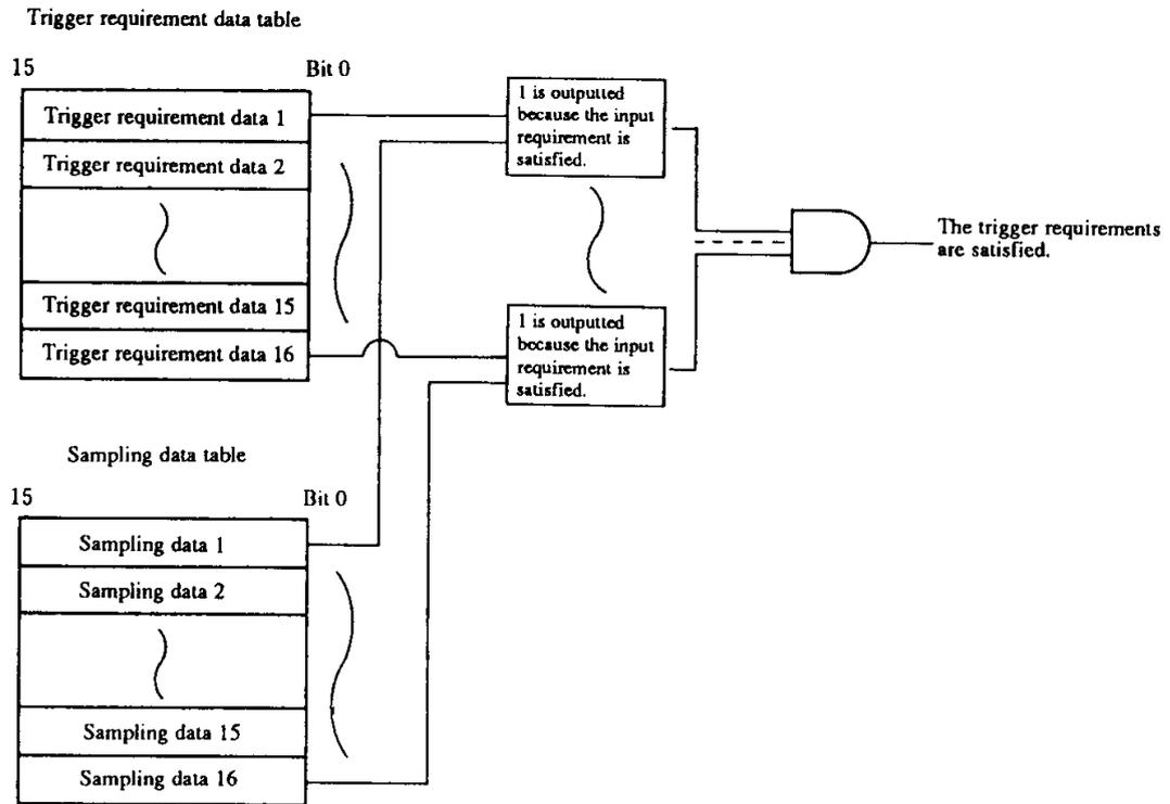
The trigger AND requirements mean that when all the trigger requirement data which is set in each I/O matches with all the I/O sampling data, the trigger requirements are satisfied.
