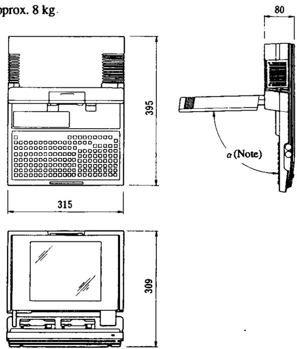
(Note) The display opening angle  $\alpha$  is 0 to 130 degrees.
