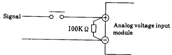
Set the input voltage within the range defined by the specifications. An excessive input may cause a serious affect onto data of other channels.
