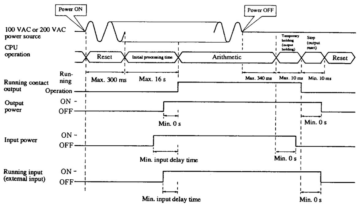
**Figure 13.1 Operation when Power is turned ON or OFF**
