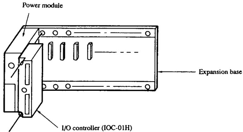
**Figure 12.5 How to mount the I/O controller**
