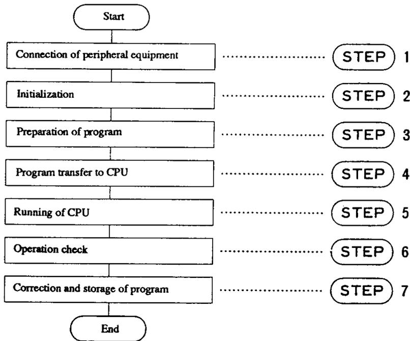
An example using the graphic programming console and HILDRL as peripheral equipment will be described. For further details, refer to the manuals (instruction manuals) of graphic programming console, portable graphic programmer, and command programmer.
