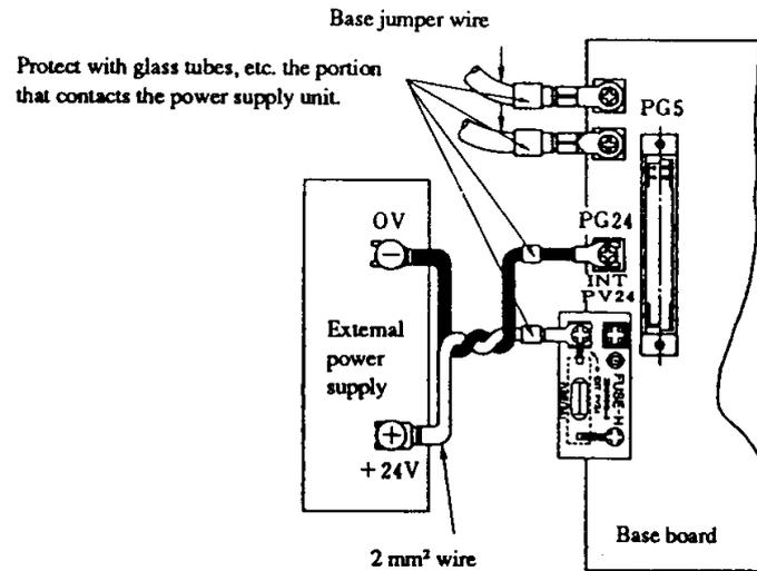
**Figure 12.2 External Power Supply Connection Diagram**
