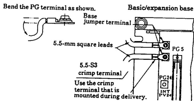
These terminals are used for base-to-base jumper lines only. Never use the terminals for signal transmission.
