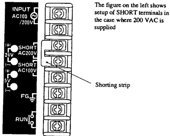
Power supply module terminal name plate
