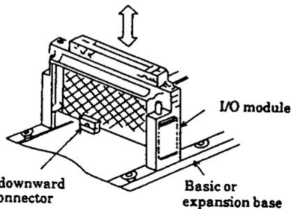
Press the module downward by engaging the connector with the socket.
