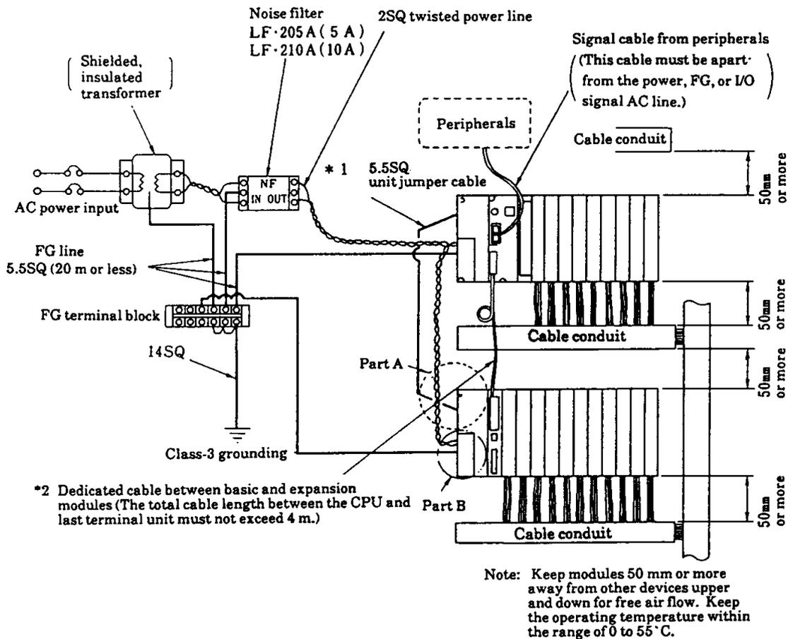
**Reference:** When the grounding cable is more than 20 m in length or connected to a common grounding terminal
