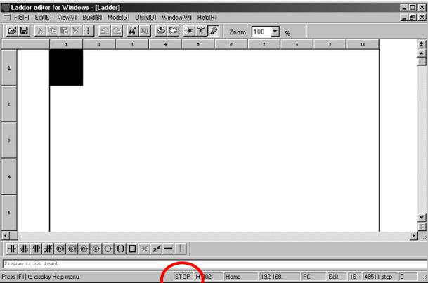
When you are on-line, an indication stating the operation condition of EH-WD10DR (RUN or STOP) appears as shown in the red circle in the left illustration.
