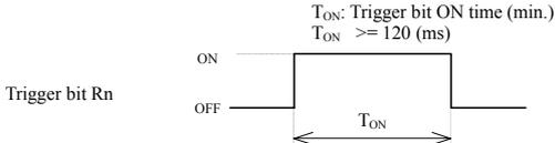
Figure 10.7 I/O Set/Reset Trigger
