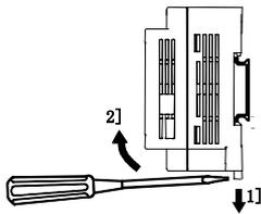
Removing from the DIN rail
