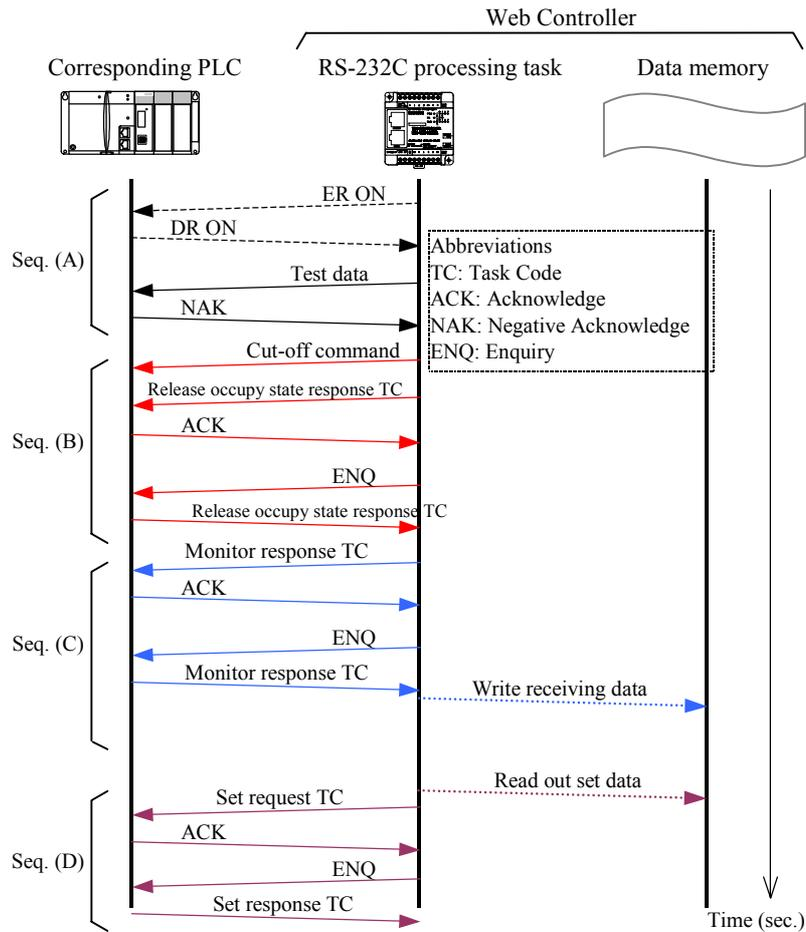
Figure 10.9 Sequence on the data link communication mode
