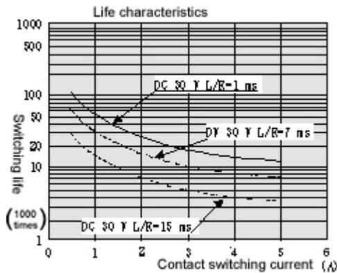
Life of the contact is almost in inverse proportion to the square of the current, so be aware that interrupting rush current or directly driving the condenser load will considerably reduce the life of the relay.
