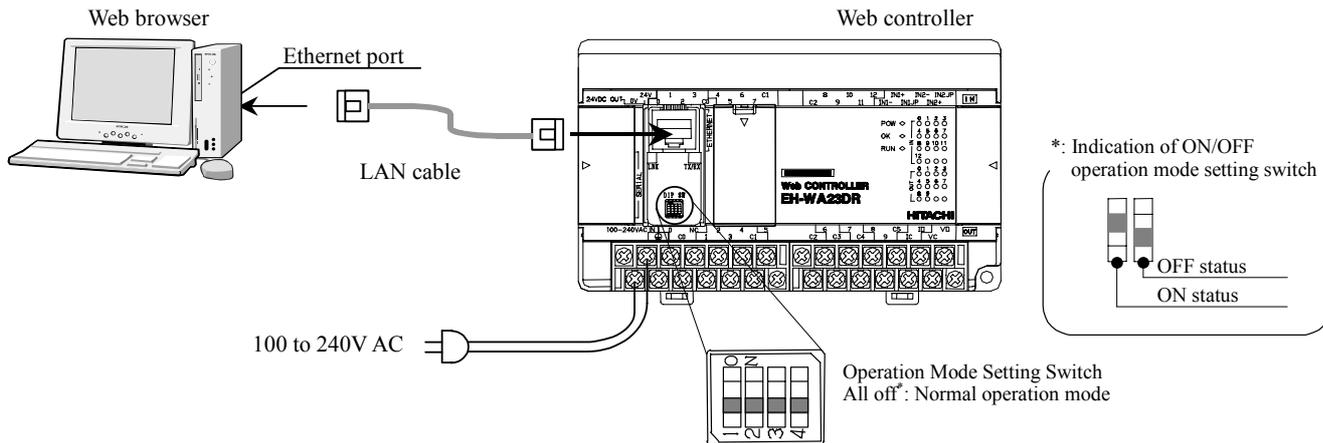
Figure0.1 Operation Mode Setting Switch (23 points type)
