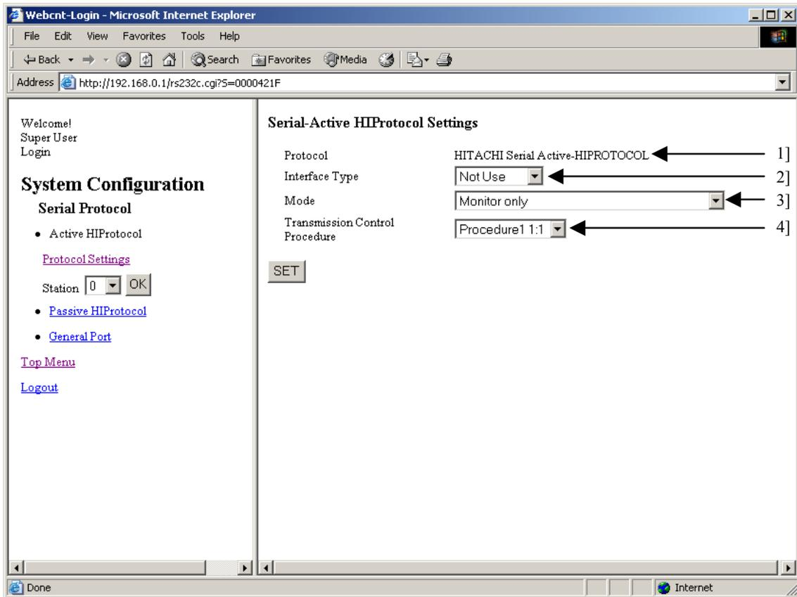
Figure 13.53 Serial Protocol - Active HIProtocol menu screen
