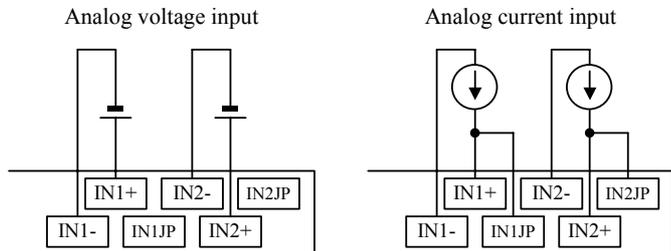
Select current or voltage type by using system configuration.
