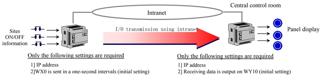
Figure 1.23 I/O transmission via Ethernet
