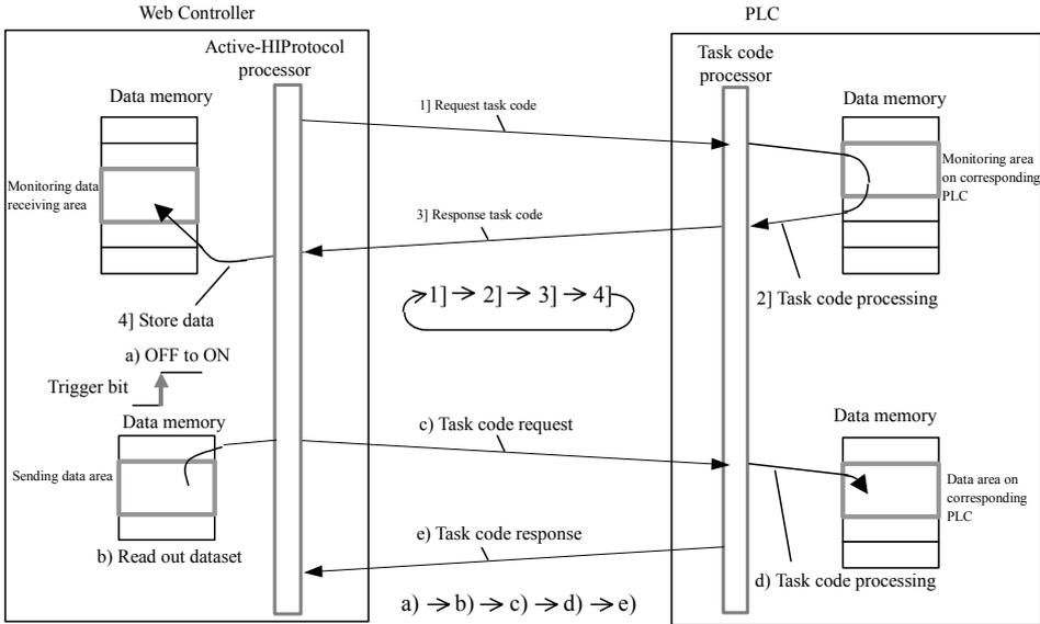
Figure 10.6 Active- HIProtocol Monitor & I/O Set/Reset Trigger
