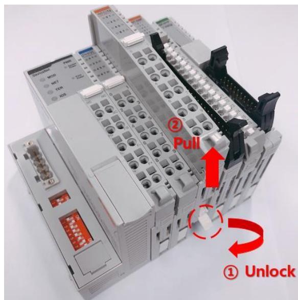
As above figure in order to safeguard the RIO3 module from jamming, it should be fixed onto the DIN rail with locking level. To do so, fold on the upper of the locking lever. To pull out the RIO3 module, unfold the locking lever as below figure.
