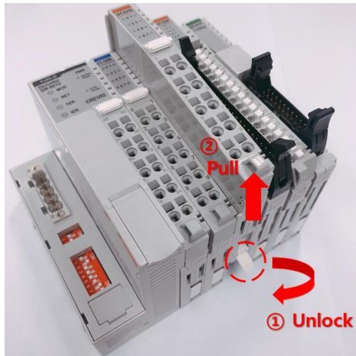
As above figure in order to safeguard the RIO3 module from jamming, it should be fixed onto the DIN rail with locking level. To do so, fold on the upper of the locking lever.
