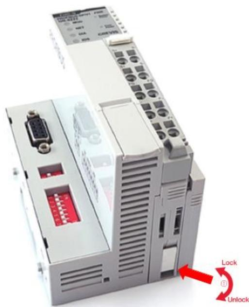
As above figure in order to safeguard the RIO3 module from jamming, it should be fixed onto the DIN rail with locking level. To do so, fold on the upper of the locking lever.
