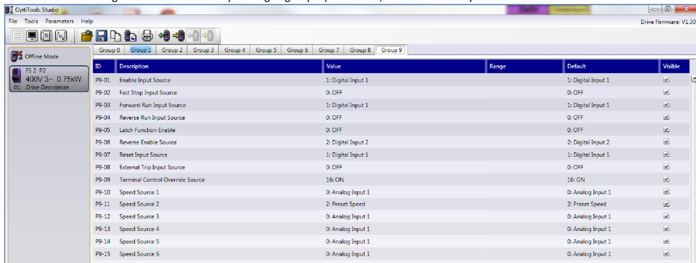
In order to 'disconnect' these internal connections, it is necessary to edit these parameters. This can only be done by setting Parameter P1-13 to 0, effectively removing the pre-defined functions in that parameter. With P1-13 set to 0, drop down options appear in group 9, and many parameter functions change:
