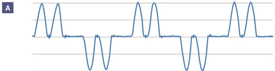
**Fig. 3** Typical current waveform characteristic at circuit point 'A' in Fig. 1
