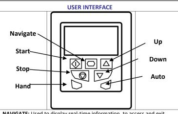
**NAVIGATE:** Used to display real-time information, to access and exit parameter edit mode and to store parameter changes
