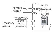
Connection diagram using terminal 2 (4 to 20mADC)
