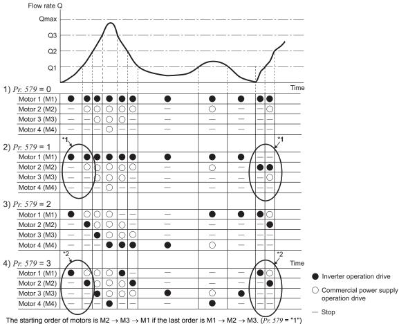
\*1 The starting order of motors is  $M2 \rightarrow M3 \rightarrow M1$  if the last order is  $M1 \rightarrow M2 \rightarrow M3$ . ( $\overline{Pr}$ , 579 = "1") \*2 The motor status in the order of elapsed time after the last inverter driving completion, from the longest (has not inverter-driven for the longest
