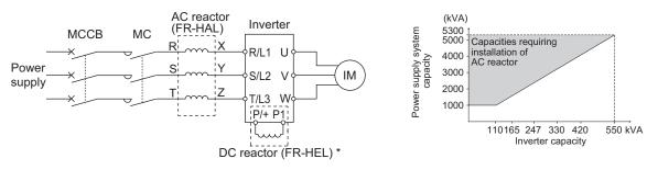
\* When connecting the FR-HEL to the 01160 or less, remove the jumper across terminals P/+ - P1. For the 01800 or more, a DC reactor is supplied. Always install the reactor.
