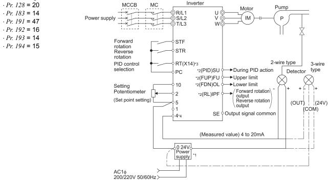
\*1 The power supply must be selected in accordance with the power specifications of the detector used.
