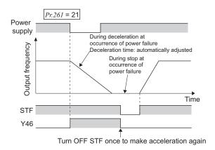
Deceleration time is automatically adjusted to keep (DC bus) voltage constant in the converter when the inverter decelerates to a stop. Even if power is restored during power failure deceleration, deceleration to a stop is continued and the inverter remains stopped. To restart, turn OFF the start signal once, then turn it ON again.
