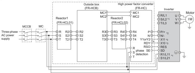
\*1 Remove the jumpers across the inverter terminals R/L1-R1/L11, S/L2-S1/L21, and connect the control circuit power supply to the R1/L11 and S1/ L21 terminals. Always keep the power input terminals R/L1, S/L2, T/L3 open. Incorrect connection will damage the inverter. (E.OPT (option fault) will occur. (*Refer to page 278.*))
