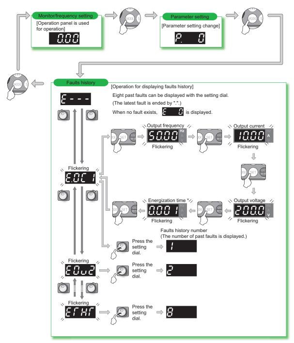
\* The cumulative energization time and actual operation time are accumulated from 0 to 65535 hours, then cleared, and accumulated again from 0. When the operation panel (FR-DU07) is used, the time is displayed up to 65.53 (65530h) in the indication of 1h = 0.001, and thereafter, it is added up from 0.
