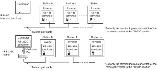
\*Set only the terminating resistor switch of the remotest inverter to the " $100\Omega$ " position.
