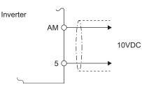
Terminal AM is factory-set to provide a 10VDC output in the full-scale status of the corresponding monitor item. Calibration parameter C1 (Pr. 901) allows the output voltage ratios (gains) to be adjusted according to the meter scale. Note that the maximum output voltage is 10VDC.
