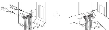
2) Using care not to bend the pins of the inverter's control circuit connector, reinstall the control circuit terminal block and fix it with the mounting screws.
