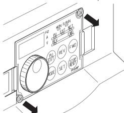
2) Push the left and right hooks of the operation panel and pull the operation panel toward you to remove.
