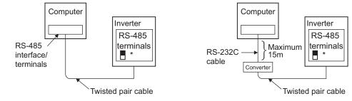
\*Set the terminating resistor switch to the "100 $\Omega$ " position.
