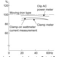
Example of measuring Inverter Output Current
