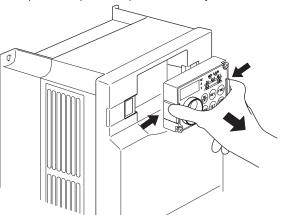
When reinstalling the operation panel, insert it straight to reinstall securely and tighten the fixed screws of the operation panel.
