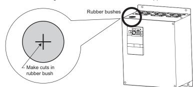
2) Insert a connector on the MT-BU5 side through a rubber bush to connect to a connector on the inverter side.
