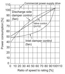
• From the motor capacity set in *Pr. 893* and *Pr. 892 Load factor*, the power estimated value (kW) during commercial power supply operation is found by the following formula.
