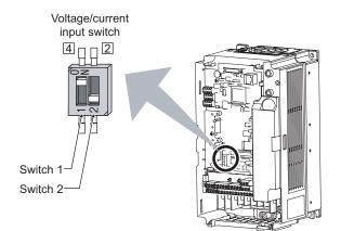
Switch 1:Terminal 4 input ON: Current input (initial status) OFF: Voltage input
