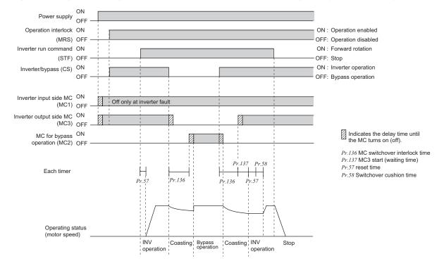
· Operation sequence example when there is automatic switchover sequence (*Pr. 139*  $\neq$  "9999", *Pr. 159* = "9999")
