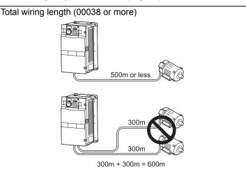
When driving a 400V class motor by the inverter, surge voltages attributable to the wiring constants may occur at the motor terminals, deteriorating the insulation of the motor. Refer to *page 46* for measures against deteriorated insulation.
