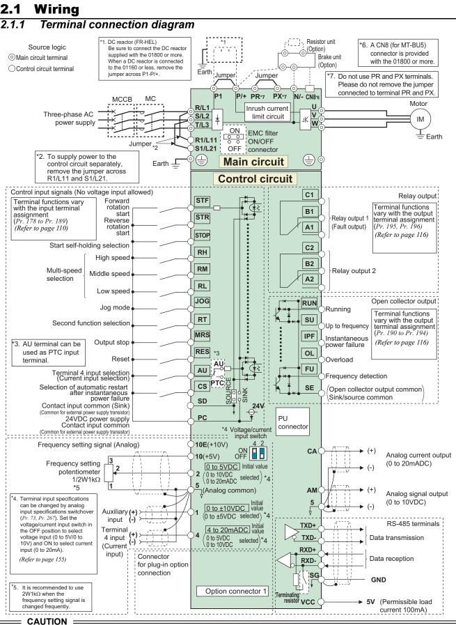
To prevent a malfunction due to noise, keep the signal cables more than 10cm away from the power cables. Also separate the main circuit wire of the input side and the output side.
