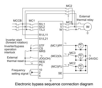
\*1 Take caution for the capacity of the sequence output terminal. The used terminal changes depending on the setting of *Pr. 190 to Pr. 196 (output terminal function selection).*
