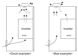
Placement of ventilation fan and inverter
