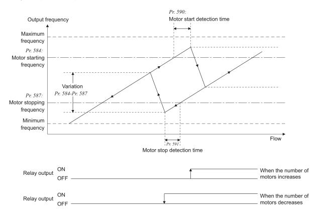
· Switchover timing at a start (stop) of an auxiliary motor 1 in the direct system (*Pr.* 579 = "2") and alternative-direct system (*Pr.* 579 = "3").
