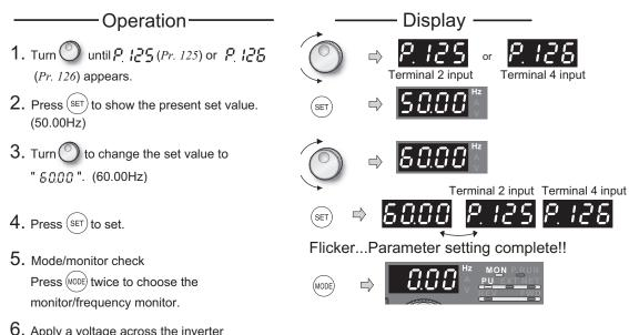
Apply a voltage across the inverter terminals 2-5 (across 4-5) and turn on the start command (STF, STR).
