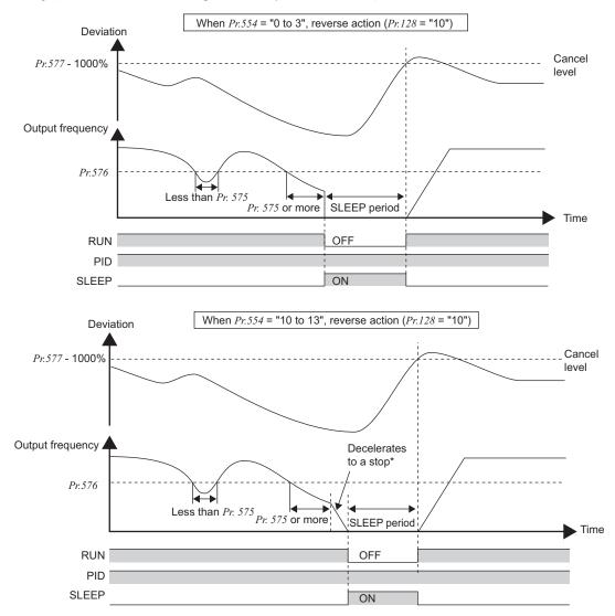
\* When the output rises to the output interruption cancel level during deceleration to a stop, output interruption gets cancelled, and the inverter accelerates again to continue PID control. *Pr.576 Output interruption detection level* is invalid during deceleration.
