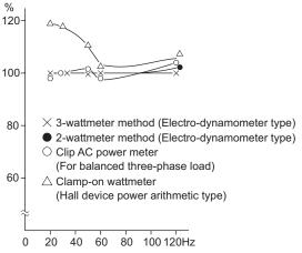
Example of measuring inverter output power
