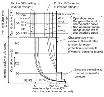
This function detects the overload (overheat) of the motor and the inverter trips. (The operation characteristic is shown on the left)
