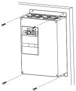
Fix six positions for the FR-F740-04320 to 08660 and fix eight positions for the FR-F740-09620 to 12120.
