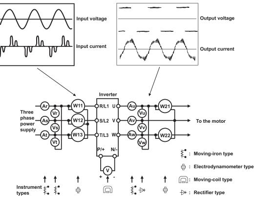
**Examples of Measuring Points and Instruments**
