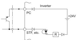
External signal input using transistor
