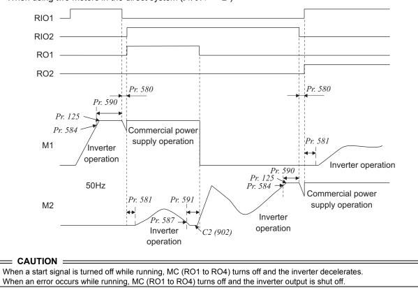
• When using two motors in the direct system (*Pr.* 597 = "2")
