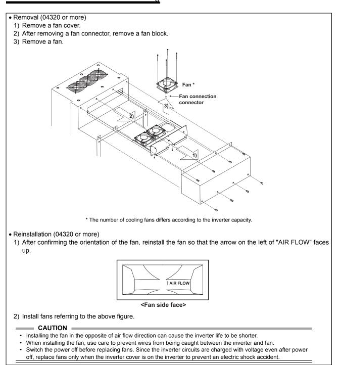
(2) Replacement procedure of the cooling fan when using a heatsink protrusion attachment (FR-A7CN)
