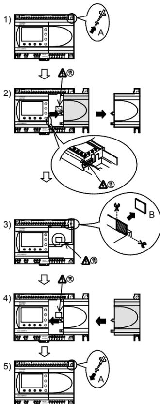
**ENG** When installing the analog module, refer to figure 2.
