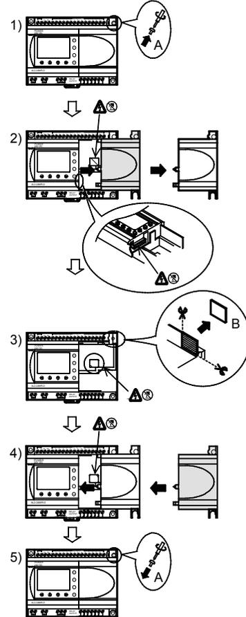
ENG When installing the analog module, refer to figure 2.
