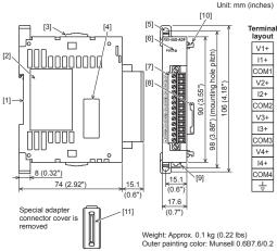
[1] DIN rail mounting groove (DIN rail: DIN46277, 35 mm (1.38") wide)
