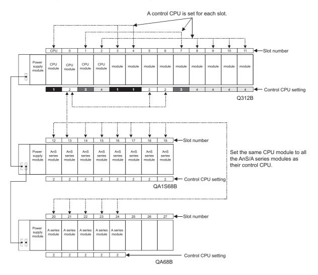
The control CPU setting shown above indicates the following:CPU modules 1 to 4:CPU numberOther than CPU modules:Control CPU number
