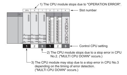
Because of this, CPU No. different from the one of the first error CPU module may be stored in the common error information field. To restore the system, eliminate the error cause of the CPU module that has been stopped by an error other than "MULTI CPU DOWN".
