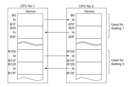
Devices of Setting 1 to 4 can be set independently for each CPU module.
