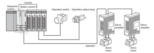
Interaction with Motion CPUs for motion control is enhanced in Universal model QCPUs.
