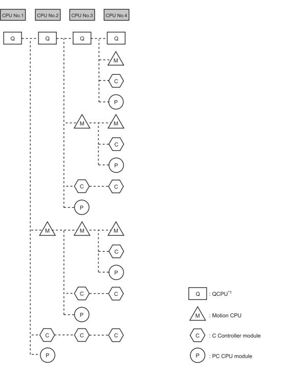
\*1 The QCPU used as CPU No.1 indicates a High Performance model QCPU or Process CPU. The QCPU used as CPU No.2 or later indicates a High Performance model QCPU, Process CPU, or Universal model QCPU (except the Q00UCPU, Q01UCPU, and Q02UCPU).
