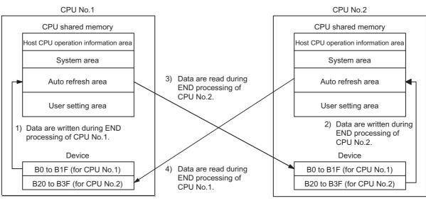
Processing performed during END processing of CPU No.1
