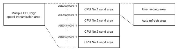
\*1 These addresses are used to specify the user setting area of the target CPU module in the cyclic transmission area device.
