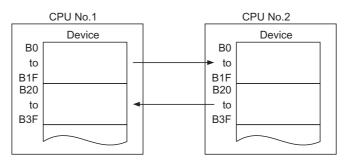
The auto refresh area in the CPU shared memory occupies a total points set for Setting 1 to 4. When the number of send points is set, the corresponding start and end addresses of the auto refresh area are automatically displayed in hexadecimal offset values.
