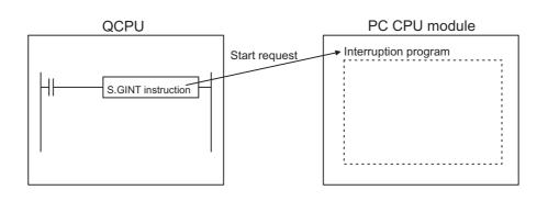
The Universal model QCPU can read/write device data from/to another Universal model QCPU by executing the multiple CPU high-speed transmission dedicated instructions listed below.
