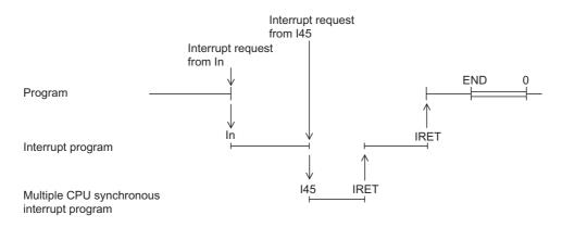
(4) Operation when an interrupt factor occurs and restrictions on programming
