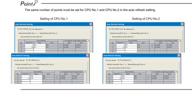
The user setting area will be 3E0\G10000 and later for CPU No.1 and 3E1\G10000 and later for CPU No.2.
