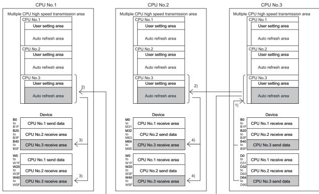
1) Data are written during END processing of CPU No.3. 2) Data are sent from CPU No.3 to CPU No.1 and No.2.
