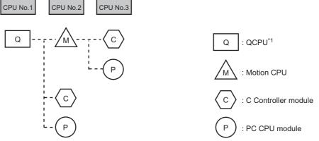
\*1 The QCPU indicates the Q00UCPU, Q01UCPU, or Q02UCPU.
