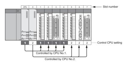
Set control CPUs in PLC parameter ("I/O Assignment").
