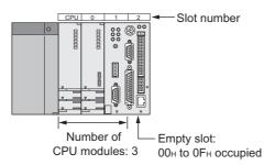
Note that the start I/O number can be changed to " $00_{H}$ " by setting "0 Point" to the number of points for the right slot of the PC CPU module in PLC parameter ("I/O Assignment").
