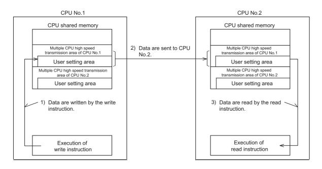
Procedure for CPU No.2 to read device data of CPU No.1
