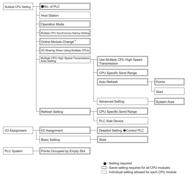
\*1 Universal model QCPUs do not support the online change function, but the setting is required to replace modules controlled by the Process CPU on the same base unit online.
