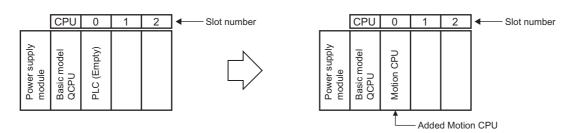
Ex. Adding a PC CPU module in slot 1 in the future
