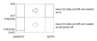
\*2 When input (X) of an output module is targeted, data are loaded as all points off.
