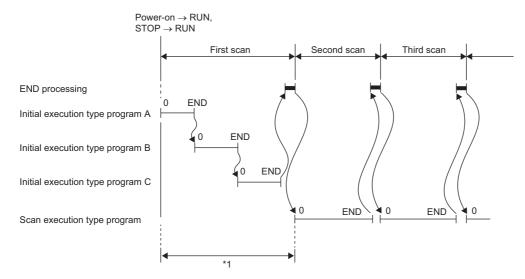
\*1 The sum of the initial execution type program execution time and END processing time is the initial scan time.
