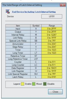
On the "Valid Range Confirmation of Latch Interval Setting" window, check the effective range for the latch timing setting. Specify the latch interval operation within the effective range.
