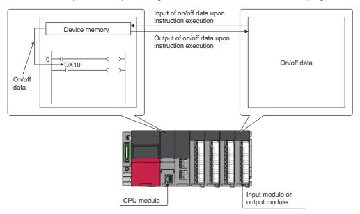
With this mode, the CPU module uses the direct access input (DX) and direct access output (DY) to perform I/O processing.
