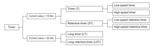
\*1 For the timer (T)/long timer (LT), the current value returns to 0 when the coil is turned off.
