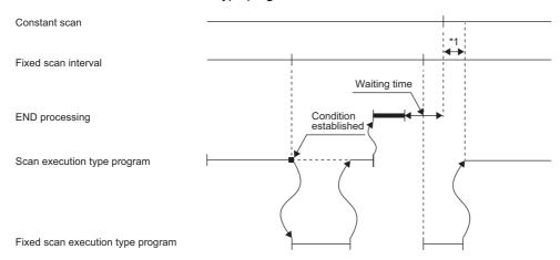
\*1 If processing does not finish during the waiting time, the scan time is extended.
