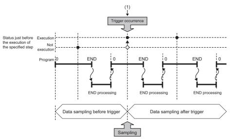
The state changes from non-running to running immediately before the execution of the specified step.
