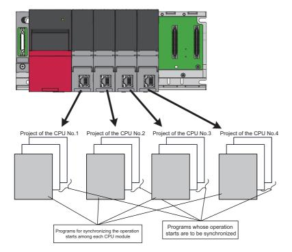
The following is an example of the configuration of a program which synchronizes the start of operation processing across CPU modules and programs which should start operation processing synchronously.
