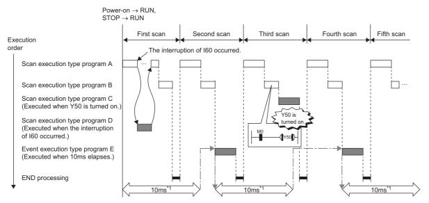
\*1 Measurement of elapsed time is 10ms or more because it is determined depending on the scan time.
