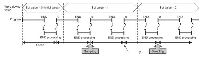
(1) The data logging function does not collect data because there has been no change in state since the last scan.
