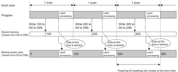
Powering off (resetting) the module at this time holds D0 to D99 = 200.
