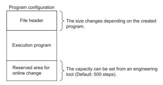
When the program is stored in the CPU module, execution program and steps reserved for online program change are allocated to the program memory. The file header is allocated to the data memory. The following table shows the destination memory to which each area is allocated when a program is stored in the CPU module.
