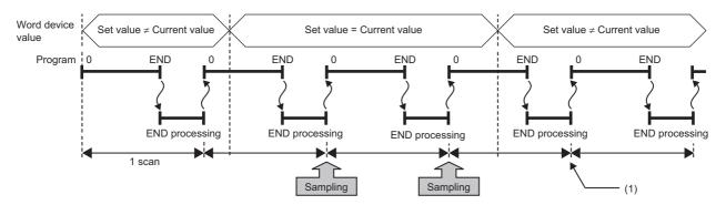
(1) During the END processing, the data logging function does not collect data because the conditions are not met.
