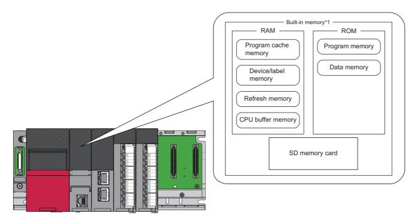
\*1 The built-in memory is a generic term of memories built in the CPU module.
