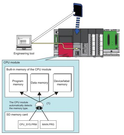
Executes the boot operation in accordance with the boot file setting when the CPU module is powered off and on or reset.
