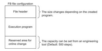
When the program memory is stored in the CPU module, execution program and steps reserved for online program change are allocated to the program memory. The file header is allocated to the data memory. The destination memory to which each area is allocated when an FB file is stored in the CPU module is the same as that for programs.
