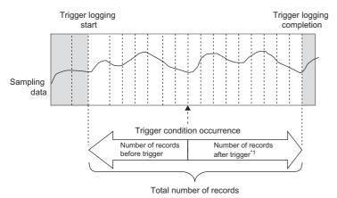
\*1 This number includes the record exactly at the time when the trigger condition is met.
