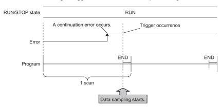
In the following situations, the occurrence of a continuation error that is specified as a trigger condition is not recognized as a trigger, with no data collection:
