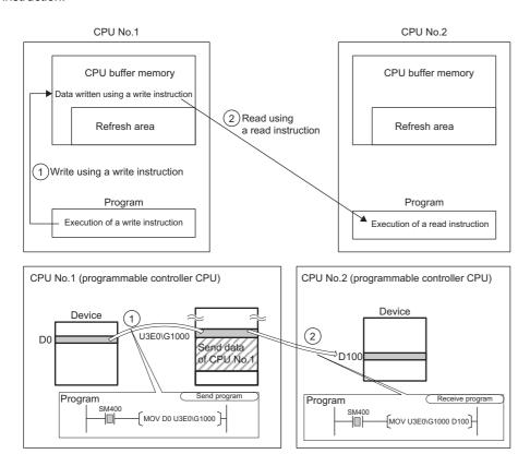
· When using an area within the fixed scan communication area
