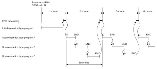
When multiple scan execution type programs are executed, the execution time of the scan execution type program will be the total time until all the scan execution type programs finish execution. Note that if interrupt program, fixed execution type program, and/or event execution type program are executed before the scan execution type program finishes execution, the execution time for these programs is also included.
