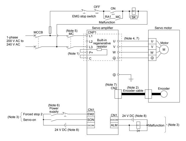
Note 1. MR-JE-40A and MR-JE-70A have a built-in regenerative resistor. (factory-wired) When using the regenerative option, refer to section 11.2.
