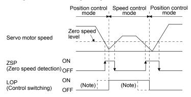
Note. When ZSP is not turned on, the control mode is not switched even if LOP is turned on/off. After LOP is turned on/off, even if ZSP is turned on, the control mode is not switched
