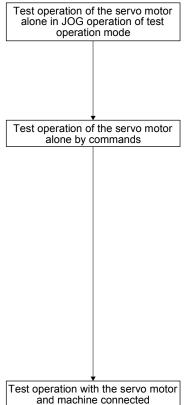
In this step, confirm that the servo amplifier and servo motor operate normally.
