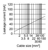
Fig. 11.2 Example of leakage current per km (lg1, lg2) for CV cable run in metal conduit
