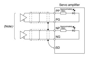
Note. Pulse train input interface is comprised of a photocoupler.
