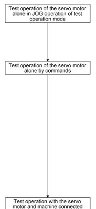
In this step, confirm that the servo amplifier and servo motor operate normally.
