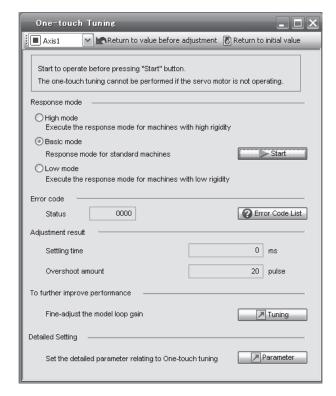
When clearing one-touch tuning is completed, the following window will be displayed. (returning to initial value)
