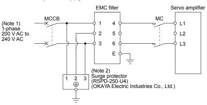
Note 1. Connect the power supply to L1 and L3. Leave L2 open.
