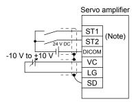
Note. This diagram shows sink I/O interface. For source I/O interface, refer to section 3.9.3.
