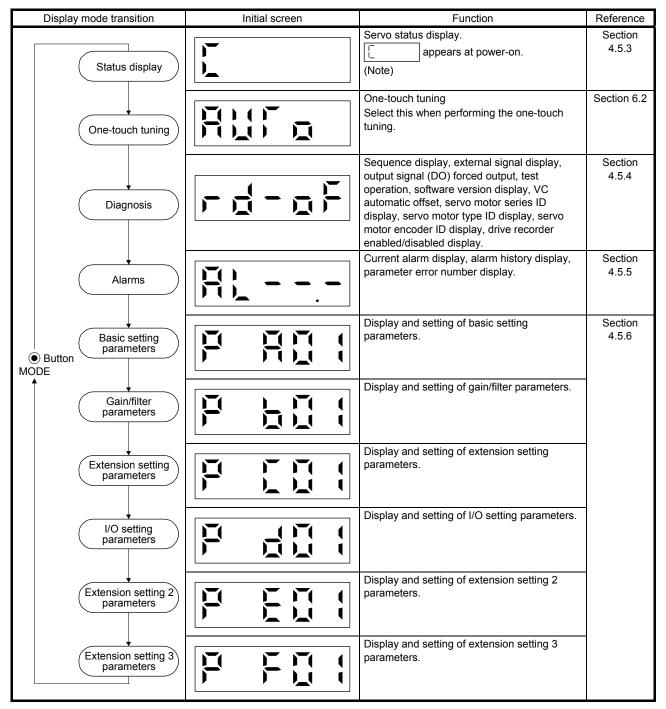
Note. When the axis name is set to the servo amplifier using MR Configurator2, the axis name is displayed and the servo status is then displayed.
