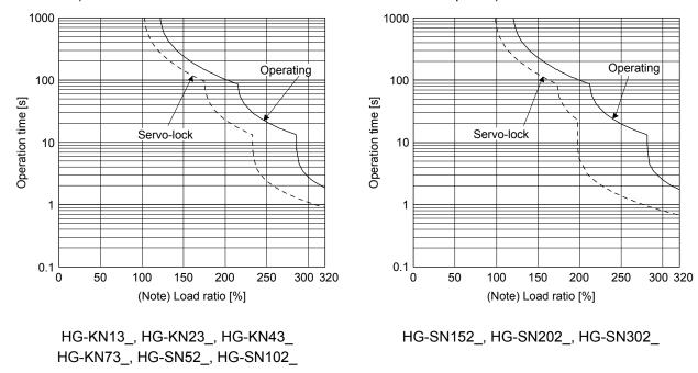
Note. If operation that generates torque more than 100% of the rating is performed with an abnormally high frequency in a servo motor stop status (servo-lock status) or in a 30 r/min or less low-speed operation status, the servo amplifier may malfunction regardless of the electronic thermal protection.
