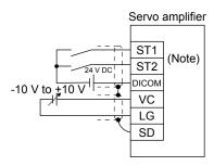
Note. This diagram shows sink I/O interface. For source I/O interface, refer to section 3.9.3.
