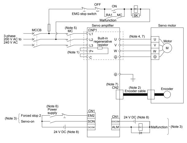
Note 1. MR-JE-40A to MR-JE-100A have a built-in regenerative resistor. (factory-wired) When using the regenerative option, refer to section 11.2.
