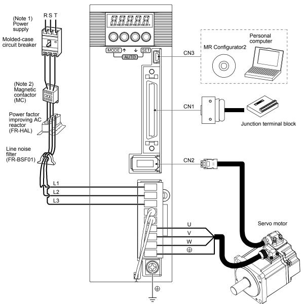
Note 1. A 1-phase 200 V AC to 240 V AC power supply may be used with the servo amplifier of MR-JE-70A or less. For 1-phase 200 V AC to 240 V AC, connect the power supply to L1 and L3. Leave L2 open. For the power supply specifications, refer to section 1.3.
