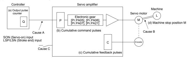
When a position shift occurs, check (a) output pulse counter Q, (b) cumulative command pulse P, (c) cumulative feedback pulse C, and (d) machine stop position M in the above diagram.
