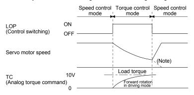
Note. When ST1 (Forward rotation start) and ST2 (Reverse rotation start) are switched off as soon as a mode is switched to the speed control, the servo motor comes to a stop according to the deceleration time constant. A shock may occur at switching control modes.
