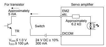
The following shows when the CN1-10 pin and the CN1-35 pin are used as digital input interface:
