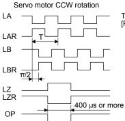
Time cycle (T) is determined by the settings of [Pr. PA15] and [Pr. PC19].
