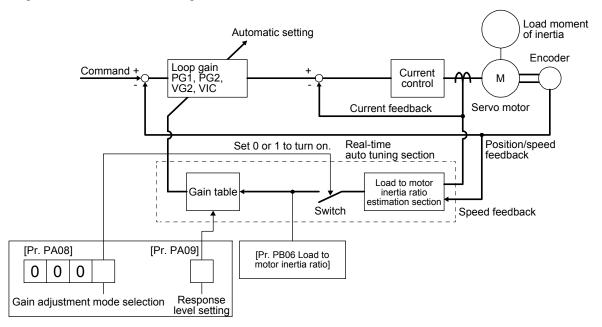
When a servo motor is accelerated/decelerated, the load to motor inertia ratio estimation section always estimates the load to motor inertia ratio from the current and speed of the servo motor. The results of estimation are written to [Pr. PB06 Load to motor inertia ratio]. These results can be confirmed on the status display screen of the MR Configurator2.
