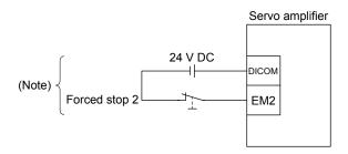
Note. This diagram shows sink I/O interface. For source I/O interface, refer to section 3.9.3.
