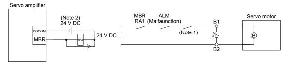
Note 1. Create the circuit in order to shut off by interlocking with the emergency stop switch.
