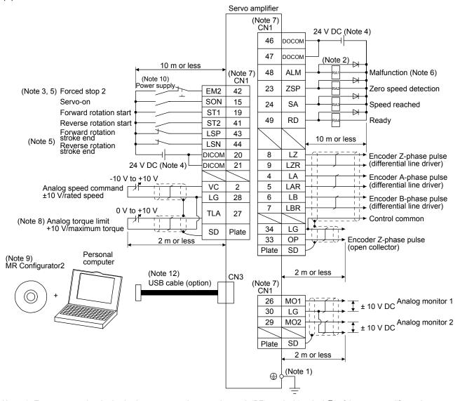
Note 1. To prevent an electric shock, always connect the protective earth (PE) terminal (marked ①) of the servo amplifier to the protective earth (PE) of the cabinet.
