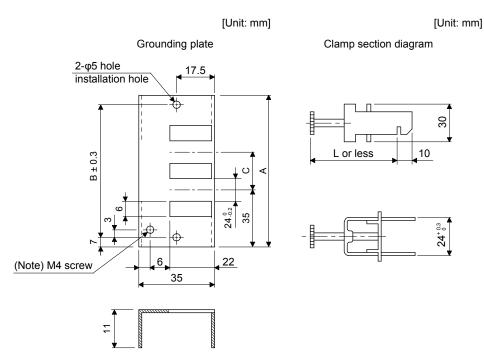
Note. Screw hole for grounding. Connect it to the grounding plate of the cabinet.
