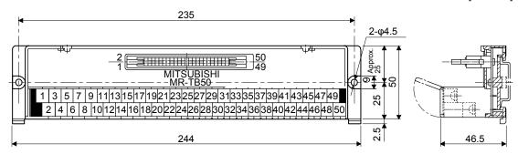
Terminal screw: M3.5 Applicable wire: 2 mm<sup>2</sup>
