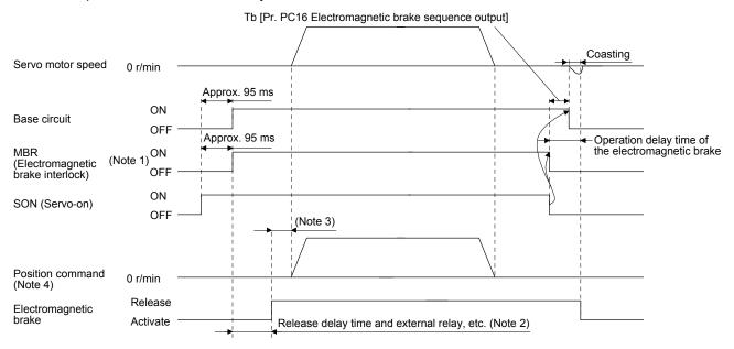
Note 1. ON: Electromagnetic brake is not activated.
