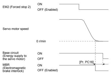
When EM2 (Forced stop 2) turns off or an alarm occurs during driving, the servo motor will decelerate based on the deceleration time constant. MBR (Electromagnetic brake interlock) will turn off, and then after the delay time set in [Pr. PC16], the servo amplifier will be base circuit shut-off status.
