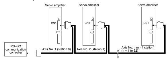
(2) Cable connection diagram Wire the cables as follows.
