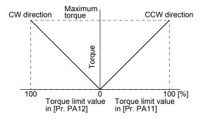
A relation between the applied voltage of TLA (Analog torque limit) and the torque limit value of the servo motor is as follows. Torque limit values will vary about 5% relative to the voltage depending on products. At the voltage of less than 0.05 V, torque may vary as it may not be limited sufficiently. Therefore, use this function at the voltage of 0.05 V or more.
