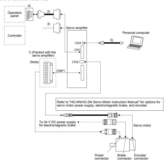
Note. Connectors for 1 kW or less. Refer to section 3.3.3 (1) (b) for 2 kW or more.
