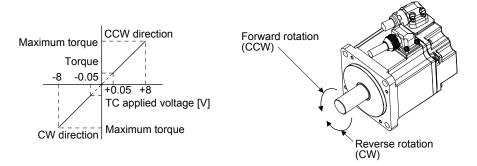
Generated torque command values will vary about 5% relative to the voltage depending on products. The torque may vary if the voltage is low (-0.05 V to 0.05 V) and the actual speed is close to the limit value. In such a case, increase the speed limit value.
