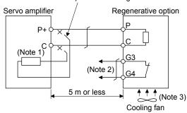
Note 1. The built-in regenerative resistor is not provided for MR-JE-10A and MR-JE-20A.
