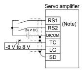
Note. This diagram shows sink I/O interface. For source I/O interface, refer to section 3.9.3.
