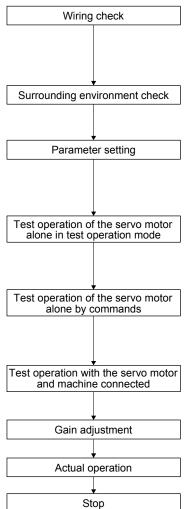
Check whether the servo amplifier and servo motor are wired correctly using visual inspection, DO forced output function (section 4.5.8), etc. (Refer to section 4.1.2.)
