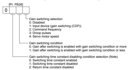
Note. This parameter setting is available with servo amplifiers with software version B4 or later.
