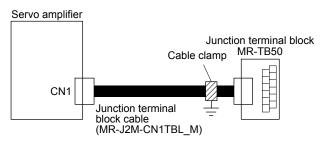
Install the junction terminal block cable on the junction terminal block side with the supplied cable clamp fitting (AERSBAN-ESET). For the use of the cable clamp fitting, refer to section 11.9, (2) (c).
