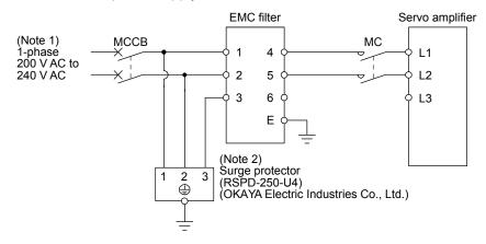
Note 1. Connect the power supply to L1 and L2. Leave L3 open.
