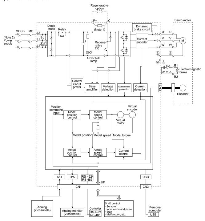
Note 1. The built-in regenerative resistor is not provided for MR-JE-10A and MR-JE-20A.
