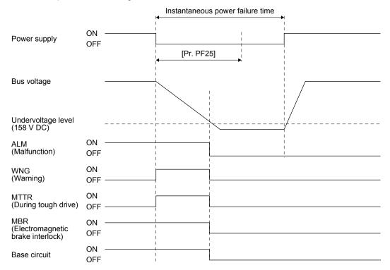
(b) When the bus voltage does not decrease lower than 158 V DC within the instantaneous power failure time
