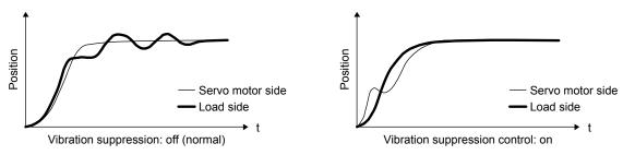
When the advanced vibration suppression control II ([Pr. PB02 Vibration suppression control tuning mode]) is executed, the vibration frequency at load side is automatically estimated to suppress machine side vibration two times at most.
