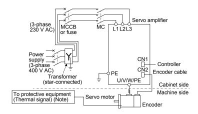
Note. Please use a thermal sensor, etc. for thermal protection of the servo motor.
