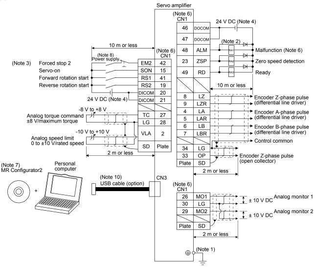
Note 1. To prevent an electric shock, always connect the protective earth (PE) terminal (marked 🚭) of the servo amplifier to the protective earth (PE) of the cabinet.
