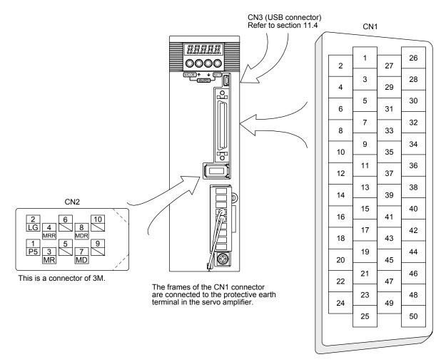
The device assignment of CN1 connector pins changes depending on the control mode. For the pins which are given parameters in the related parameter column, their devices will be changed using those parameters.
