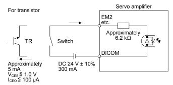
The following shows when the CN1-37 pin and the CN1-38 pin are used as digital input interface:
