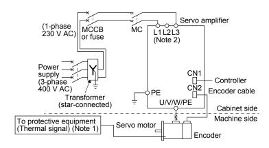
Note 1. Please use a thermal sensor, etc. for thermal protection of the servo motor.
