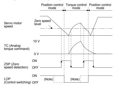
Note. When ZSP is not turned on, the control mode is not switched even if LOP is turned on/off. After LOP is turned on/off, even if ZSP is turned on, the control mode is not switched.
