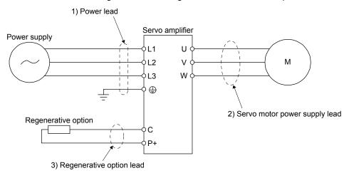
Table 11.1 shows examples for using the 600 V Grade heat-resistant polyvinyl chloride insulated wire (HIV wire).
