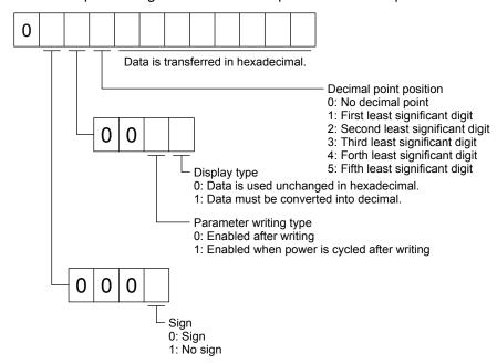
For example, data "00120000270F" means 999.9 (decimal display format) and data "00000003ABC" means 3ABC (hexadecimal display format).
