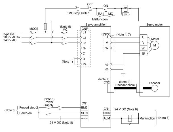
Note 1. Always connect between P+ and D terminals. (factory-wired) When using the regenerative option, refer to section 11.2.
