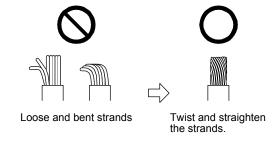
You can also use a ferrule to connect with the connectors. When you use a ferrule, use the following ferrules and crimp terminal.
