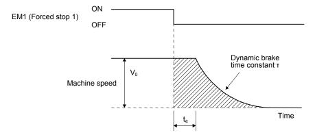
Fig. 10.3 Dynamic brake operation diagram
