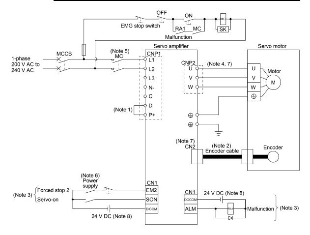
Note 1. Always connect between P+ and D terminals. (factory-wired) When using the regenerative option, refer to section 11.2.
