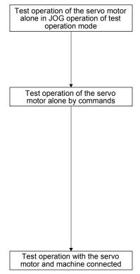
In this step, confirm that the servo amplifier and servo motor operate normally.
