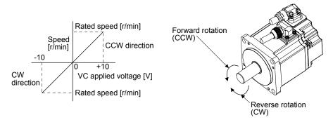
The following table indicates the rotation direction according to ST1 (Forward rotation start) and ST2 (Reverse rotation start) combination.
