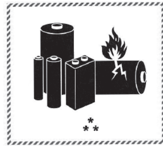
* Place for UN number (s) ** Place for telephone number for additional information Fig. app. 2 Example of Mitsubishi label with battery illustration (Available from January 1, 2017)
