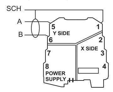
The use of screened cables is always recommended, and especially whenever the length of the connections is greater than 3 m
