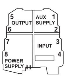
2 wires Connections Active Current Input.
