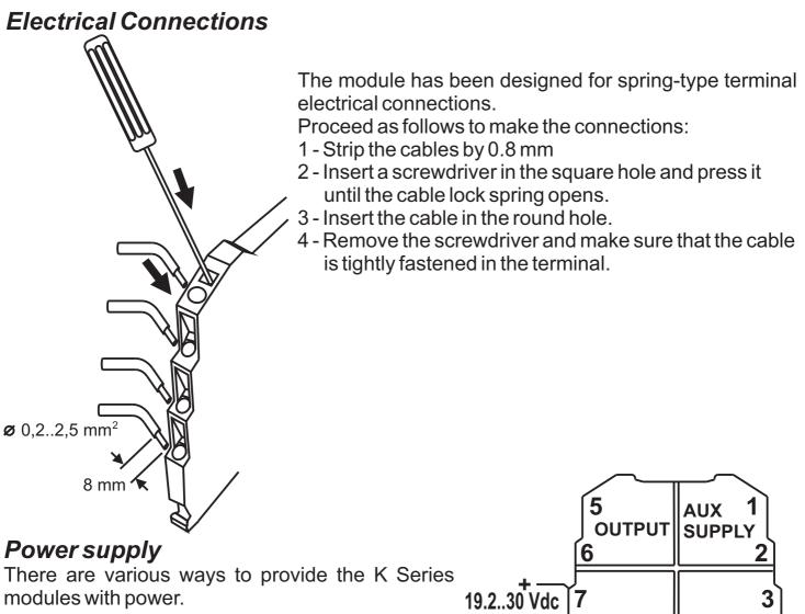
1 - Direct power supply to the modules by connecting 24 Vdc power supply directly to Terminals 7 (+) and 8 (-) of each module.
