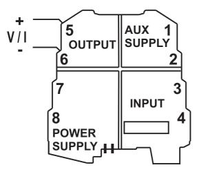
Note: in order to reduce the instrument's dissipation, we recommend either using the output for voltage or guaranteeing a load of > 250  $\Omega$  to the current output.
