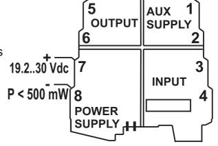
2 - Using the K-BUS connector accessory for the distribution of the power supply to the modules via bus connector, in this way eliminating the need to connect power supply to each module.
