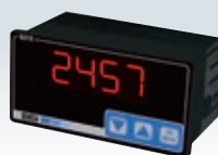
4-digit display loop powered indicator, 4-20 mA input
